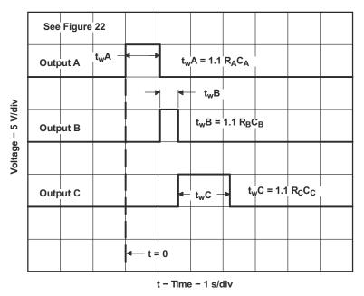
Figure 7-8. Sequential Timer Waveforms
