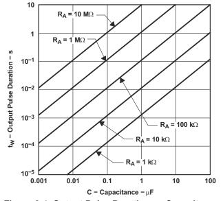
Figure 6-4. Output Pulse Duration vs Capacitance
