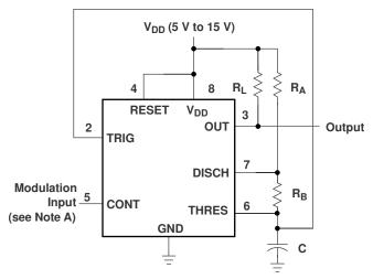
A. The modulating signal can be direct or capacitively coupled to CONT. For direct coupling, the effects of modulation source voltage and impedance on the bias of the timer must be considered.
