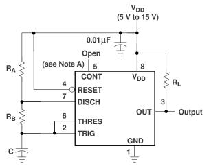
A. Decoupling CONT voltage to ground with a capacitor can improve operation. This must be evaluated for individual applications.
