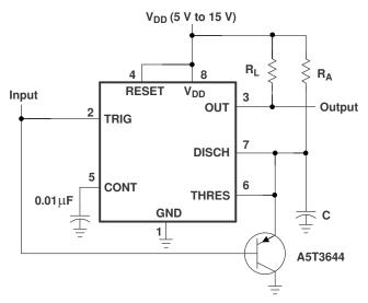
Figure 7-1. Circuit for Missing-Pulse Detector
