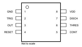
Figure 4-1. D Package, 8-Pin SOIC, (Top View)
