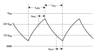
Figure 6-7. Trigger and Threshold Voltage Waveform
