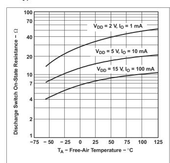
Figure 5-1. Discharge Switch ON-State Resistance vs Free-Air Temperature
