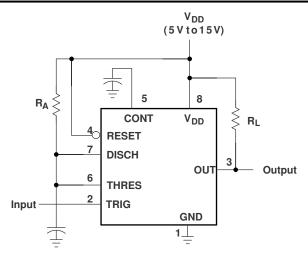
Figure 6-2. Circuit for Monostable Operation
