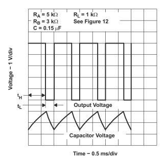
Figure 6-6. Typical Astable Waveforms
