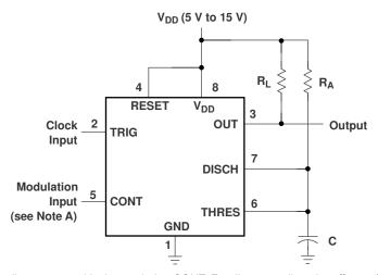
The modulating signal can be direct or capacitively coupled to CONT. For direct coupling, the effects of modulation source voltage and impedance on the bias of the timer must be considered.
