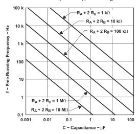
Figure 6-8. Free-Running Frequency
