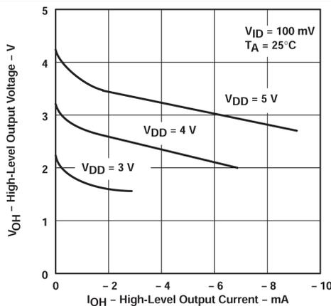
Figure 5-5. High-level Output Voltage vs High-level Output Current
