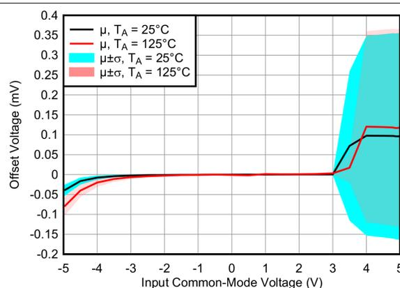
**Figure 7-4. Offset Voltage vs Input Common-mode Voltage**
