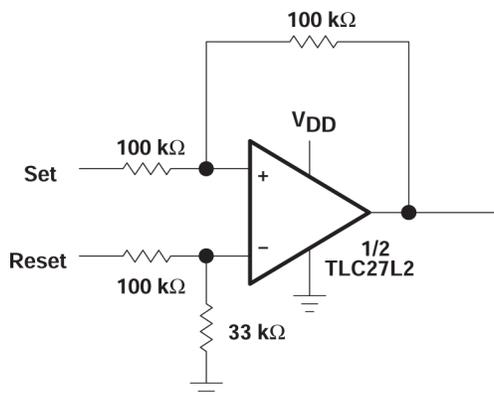
Figure 7-10. Set/Reset Flip-Flop,  $V_{DD} = 5V$  to  $12V$
