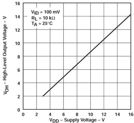
Figure 5-7. High-level Output Voltage vs Supply Voltage
