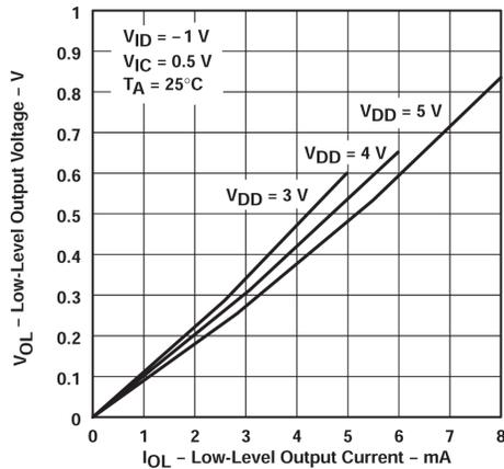
**Figure 5-13. Low-level Output Voltage vs Low-level Output Current**
