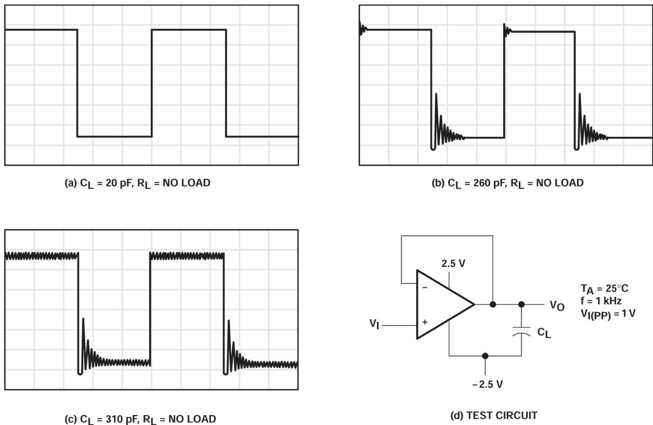
**Figure 7-7. Effect of Capacitive Loads and Test Circuit**
