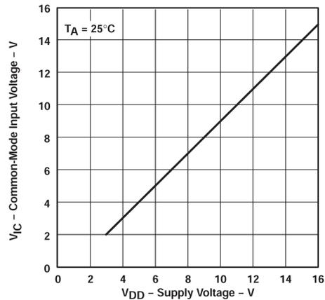
**Figure 5-18. Common-mode Input Voltage Positive Limit vs Supply Voltage**
