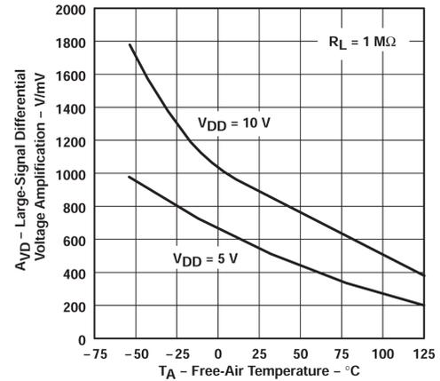
**Figure 5-16. Large-signal Differential Voltage Amplification vs Free-air Temperature**
