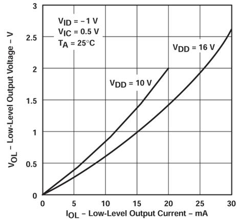
**Figure 5-14. Low-level Output Voltage vs Low-level Output Current**
