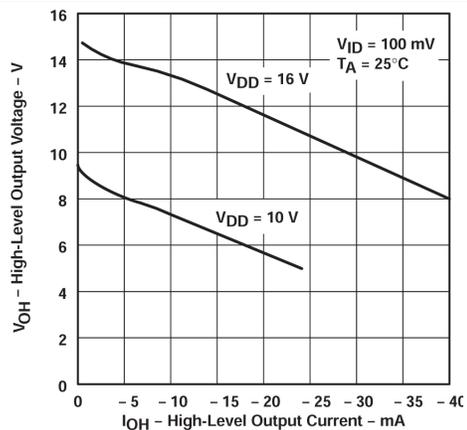
Figure 5-6. High-level Output Voltage vs High-level Output Current
