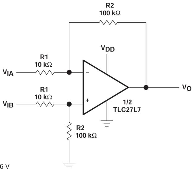
NOTE:  $V_{DD} = 5\text{ V to }16\text{ V}$
