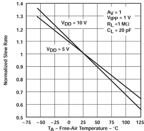
Figure 5-23. Normalized Slew Rate vs Free-air Temperature
