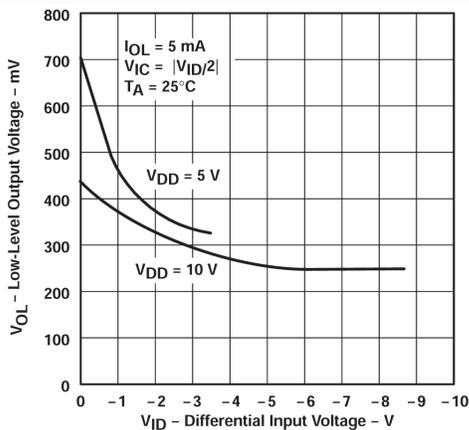
Figure 5-11. Low-level Output Voltage vs Differential Input Voltage
