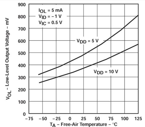
Figure 5-12. Low-level Output Voltage vs Free-air Temperature
