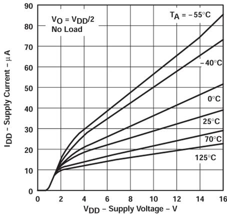
Figure 5-19. Supply Current vs Supply Voltage
