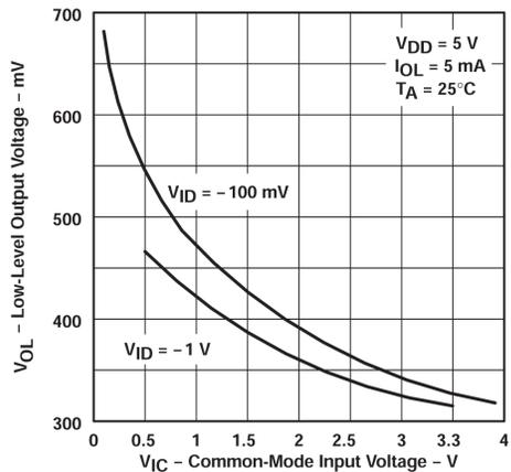
Figure 5-9. Low-level Output Voltage vs Differential Input Voltage
