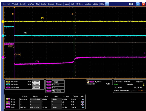
Figure 9-4. OUT In Current Fault Auto Recovery, Low Side Mode
