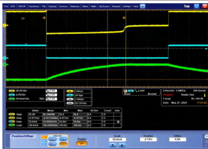
Figure 8-5. CQ Power Up Delay, t_{UVLO} (Pin mode or the default 00b setting in SPI mode)
