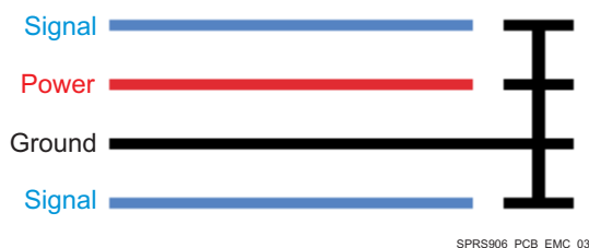
Figure 7-13. Guard Ring Routing
