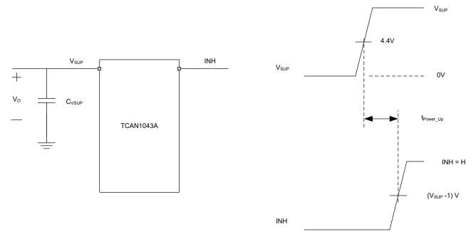
Figure 6-10. Power-Up Timing
