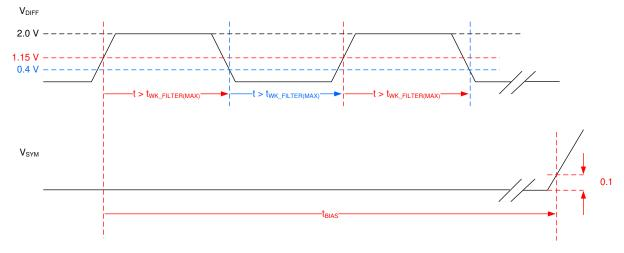
Figure 6-9. Bias Reaction Time Measurement
