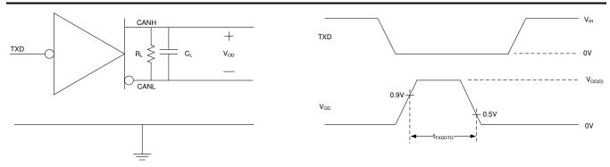
Figure 6-7. TXD Dominant Time Out Test Circuit and Measurement
