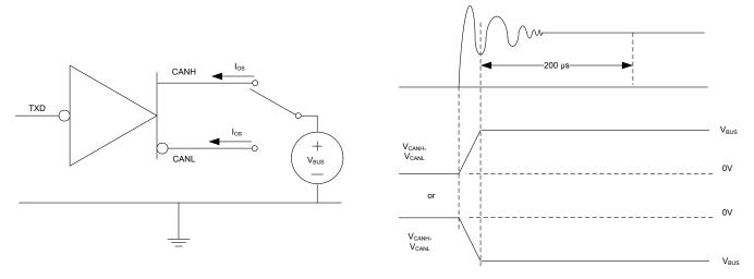
Figure 6-8. Driver Short-Circuit Current Test and Measurement
