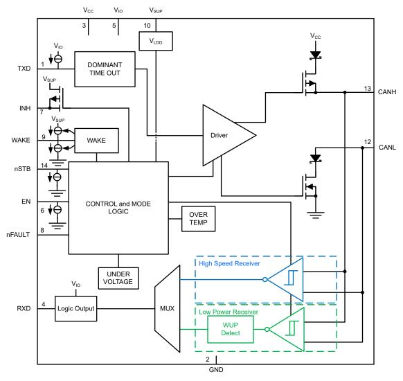
Figure 7-3. TCAN1473-Q1 Functional Block Diagram
