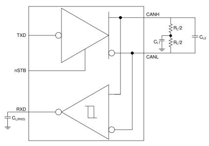
Figure 6-2. Test Circuit
