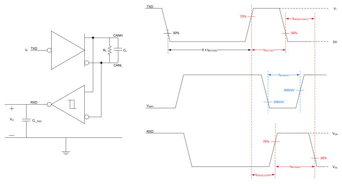
Figure 6-6. Transmitter and Receiver Timing Behavior Test Circuit and Measurement
