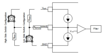
Figure 7-8. WAKE Circuit Example
