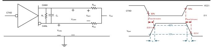
Figure 6-4. Driver Test Circuit and Measurement
