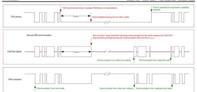
Figure 7-5. Timing Diagram for TXD DTO
