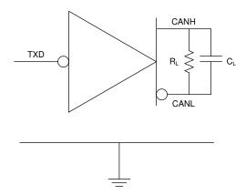
Figure 6-3. Supply Test Circuit
