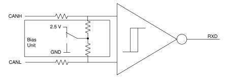
Figure 6-1. Common-Mode Bias Unit and Receiver
