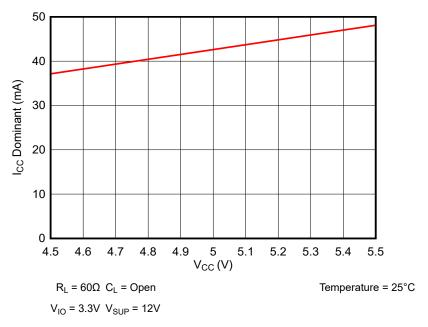
Figure 8-3. I<sub>CC</sub> Dominant over I<sub>CC</sub> Supply Voltage
