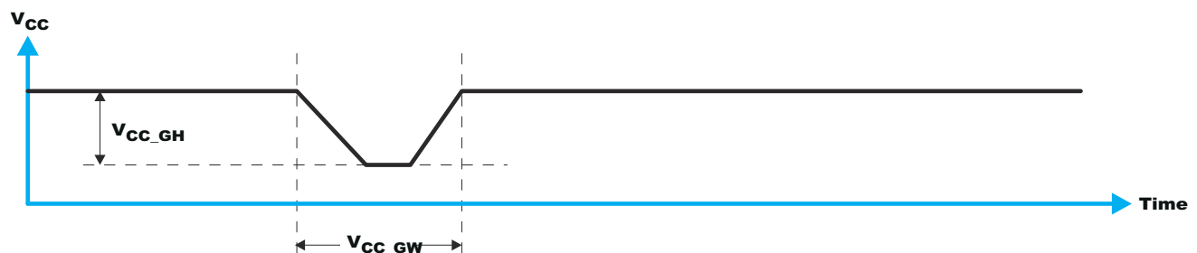
Figure 9-8. Glitch Width and Glitch Height
