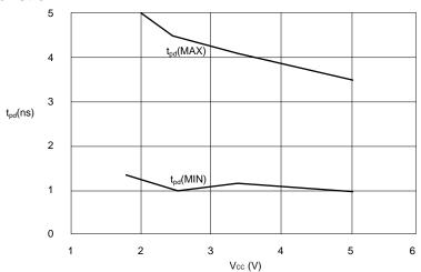
Figure 1.  $t_{pd}$  vs  $V_{CC}$
