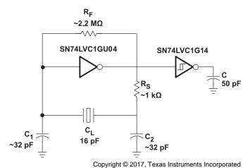
Figure 5. Typical Application Diagram
