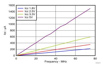
Figure 6. I<sub>CC</sub> vs Frequency
