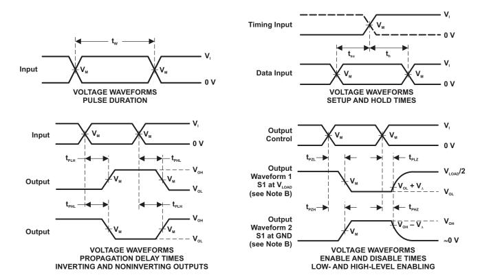
NOTES: A. C, includes probe and jig capacitance.
