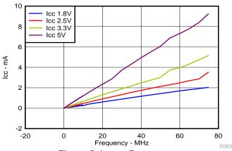
Figure 5. I<sub>CC</sub> vs Frequency
