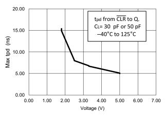
Figure 5. Max tpd vs Voltage of LVC Family
