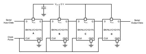
Figure 4. 4-Bit Serial Shift Register
