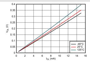
Figure 5-11. Output Voltage vs Current in LOW State; 2.5V Supply
