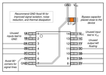
Figure 8-3. Example Layout for the SN74LVC11A
