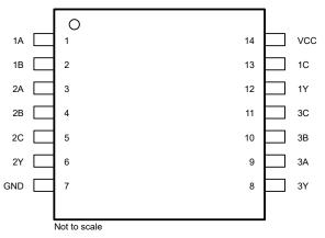
Figure 4-2. SN74LVC11A D or PW (Preview) Packages, 14-Pin SOIC or TSSOP (Top View)
