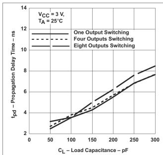
Figure 5-1. Propagation Delay (Low to High Transition)
