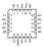
Figure 4-3. FK Package 20-Pin LCCC (Top View)
