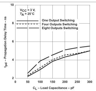
Figure 5-2. Propagation Delay (High to Low Transition)
