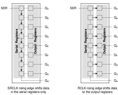
Figure 9-2. Simplified Functional Diagram Showing Clock Operation
