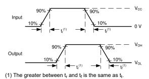
Figure 6-5. Voltage Waveforms, Input and Output Transition Times
