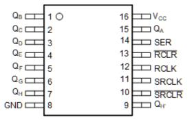
Figure 4-1. PW Package, 16-Pin TSSOP (Top View)
