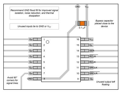
Figure 9-3. Example Layout for the SN74LV8T594 in TSSOP
