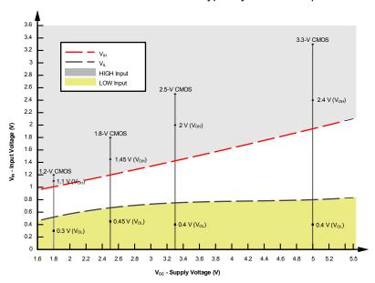
Figure 8-2. LVxT Input Voltage Levels
