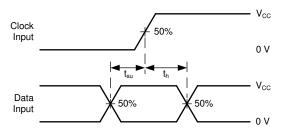
Figure 6-3. Voltage Waveforms, Setup and Hold Times
