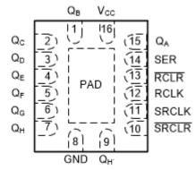
Figure 4-2. BQB Package, 16-Pin WQFN (Transparent Top View)
