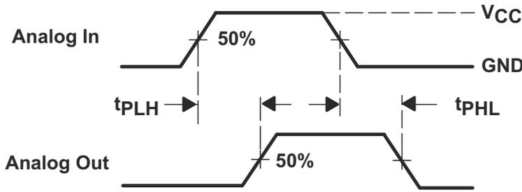
Figure 6-7. Propagation Delays, Analog In to Analog Out
