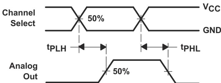
Figure 6-5. Propagation Delays, Channel Select to Analog Out
