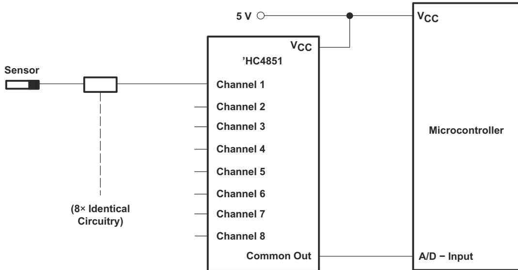
Figure 8-3. Solution by Applying the 'HC4851 Multiplexer
