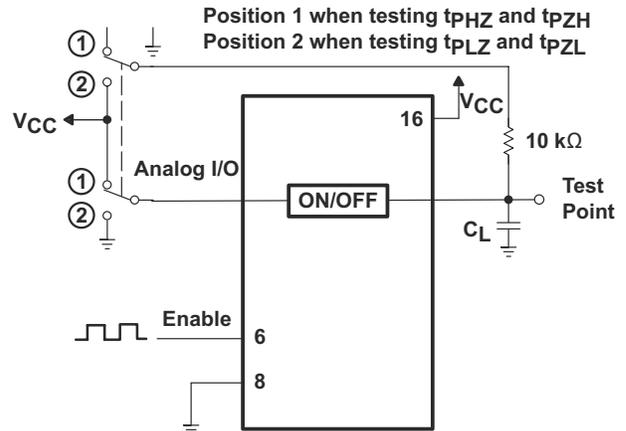
Figure 6-10. Propagation-Delay Test Setup, Enable to Analog Out
