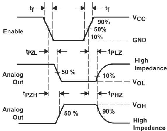
Figure 6-9. Propagation Delays, Enable to Analog Out
