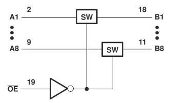
Figure 7-2. Logic Diagram (Positive Logic)
