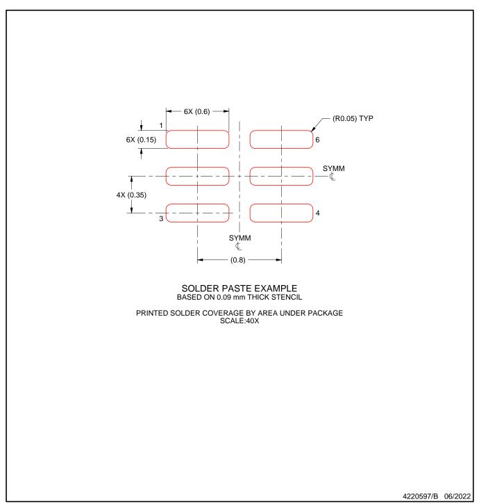
4. Laser cutting apertures with trapezoidal walls and rounded corners may offer better paste release. IPC-7525 may have alternate design recommendations.
