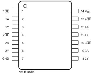
Figure 4-1. D, DB, DGV, N, NS, J, W, or PW Package 14-Pin SOIC, SSOP, TVSOP, PDIP, SO, CDIP, CFP, or TSSOP Top View
