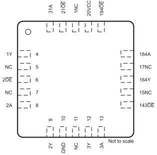
Figure 4-3. FK Package 20-Pin LCCC Top View
