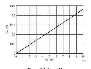
Figure 8-3.  $I_{OL}$  vs  $V_{OL}$
