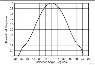
Figure 8-7. Angular Response of this FPCB Design Along the Less-Restricted Rotational Axis
