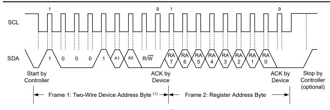
Figure 6-5. Setting the I<sup>2</sup>C Register Address
