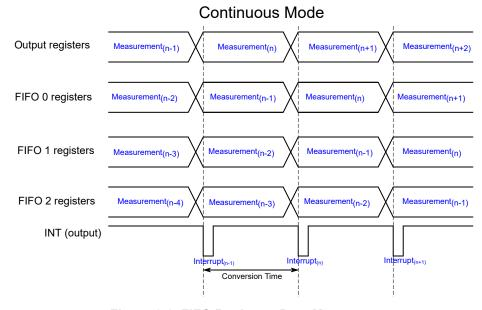
Figure 6-2. FIFO Registers Data Movement
