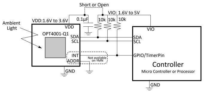
Figure 8-1. Typical Application Schematic
