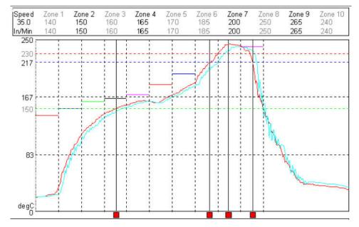
Figure 8-11. Recommended Solder Reflow Temperature Profile
