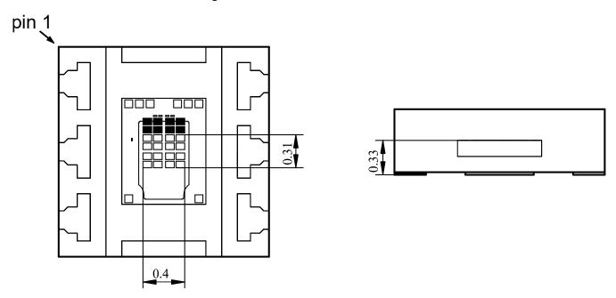
Figure 8-3. USON Sensor Position
