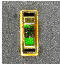
Figure 8-5. Image of FPCB With OPT4001-Q1 Mounted, Receiving Light Through the Cutout With a Rectangular Shape
