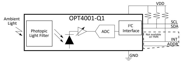
Figure 6-1. Functional Block Diagram of the OPT4001-Q1
