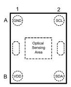
Figure 4-1. YMN Package, 4-Pin PicoStar™ (Top View)
