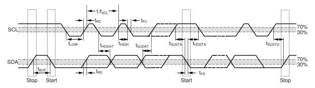
Figure 5-1. I<sup>2</sup>C Detailed Timing Diagram
