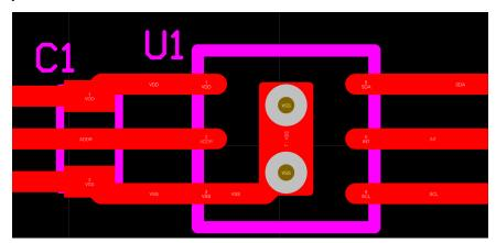
Figure 8-12. Layout Example for DNP Package
