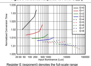
Figure 5-12. Conversion Time at 25ms vs Input Light Level
