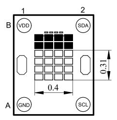
Figure 8-2. PicoStar™ Sensor Position
