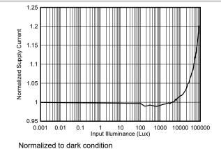
Figure 5-6. Active Current vs Input Light Level
