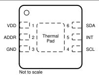
Figure 4-2. DNP Package, 6-Pin USON (Top View)
