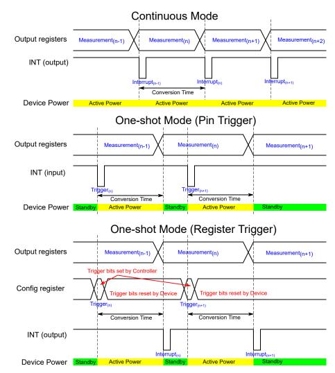
Figure 6-3. Timing Diagrams for Different Operating Modes
