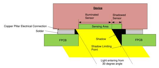
Figure 8-6. Cross-Sectional Diagram of OPT4001-Q1 Soldered to an FPCB With a Cutout, Including Light Entering From an Angle
