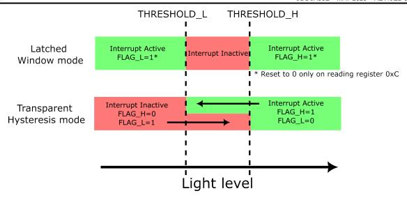
Figure 6-4. Interrupt Pin Status (INT\_CFG = 0 Setting) and Register Flag Behavior
