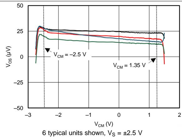
Figure 53. Input Offset Voltage vs Common-Mode Voltage
