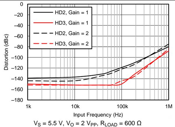
**Figure 17. Distortion vs Frequency for Various Gains**
