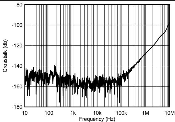
Figure 24. Crosstalk vs Frequency
