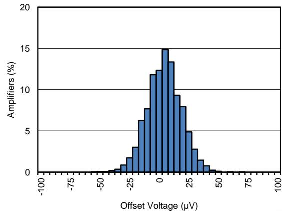
Figure 37. Input Offset Voltage Distribution
