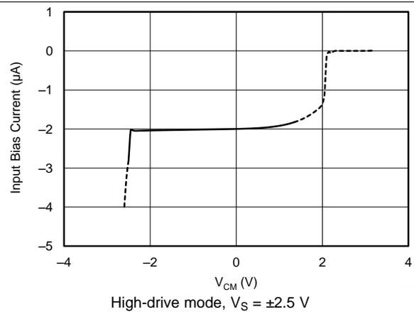
Figure 51. Input Bias Current vs Input Common-Mode Voltage
