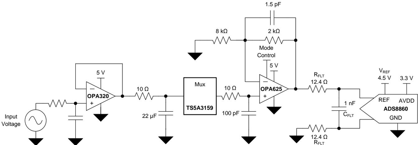
**Figure 76. Single-Supply, 16-Bit, 1-MSPS, Multiplexed, SAR ADC Driver**
