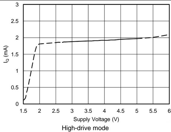
Figure 56. High-Drive Mode Quiescent Current vs Power-Supply Voltage
