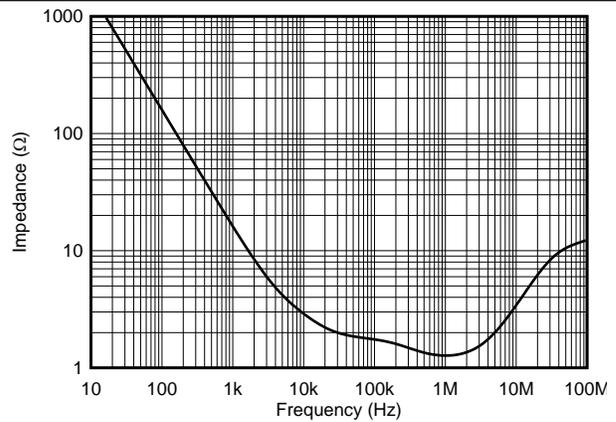
Figure 9. High-Drive Mode Open-Loop Output Impedance vs Frequency
