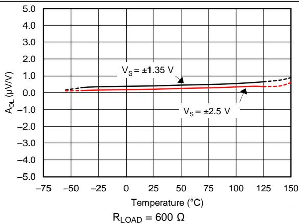
Figure 50. Open-Loop Gain vs Temperature with 600-Ω Load
