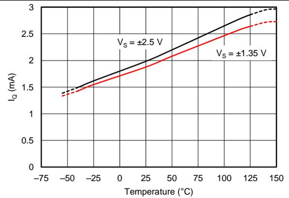
Figure 57. High-Drive Mode Quiescent Current vs Temperature
