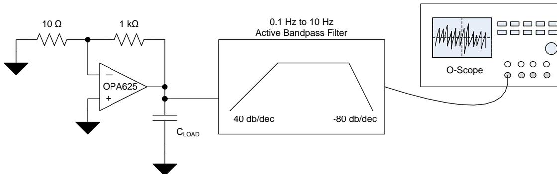
Figure 69. 0.1-Hz to 10-Hz Voltage-Noise Measurement Circuit
