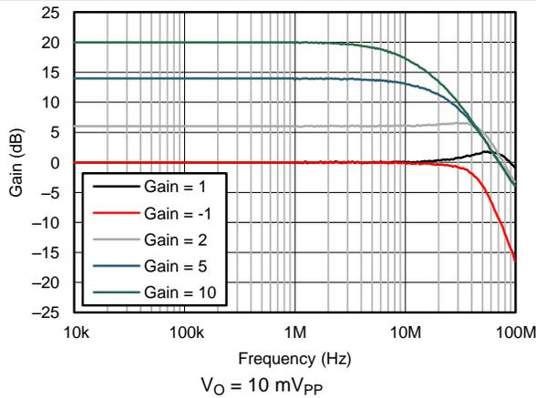
Figure 2. Small-Signal Frequency Response for Various Gains
