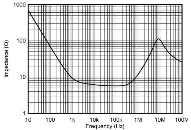
Figure 11. Low-Power Mode Open-Loop Output Impedance vs Frequency
