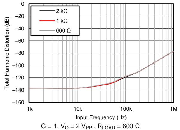
Figure 21. Total Harmonic Distortion vs Frequency for Various Loads
