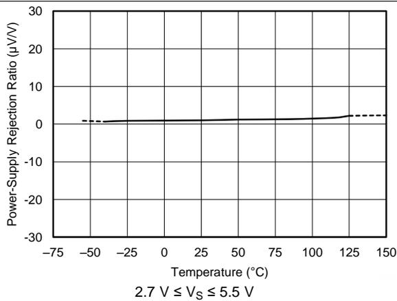
Figure 48. Power-Supply Rejection Ratio vs Temperature
