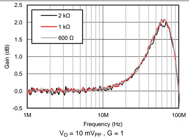
Figure 7. Small-Signal Frequency Response for Various Resistive Loads
