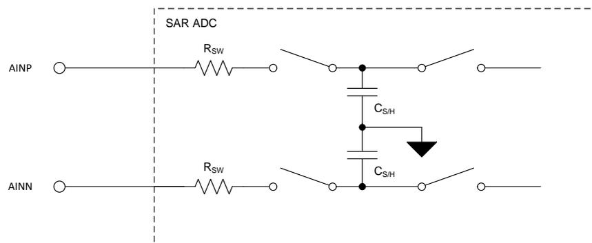
**Figure 74. Simplified SAR ADC Input**
