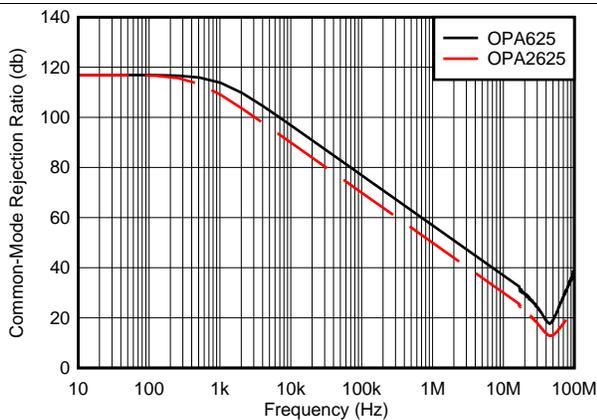
Figure 12. Common-Mode Rejection Ratio vs Frequency
