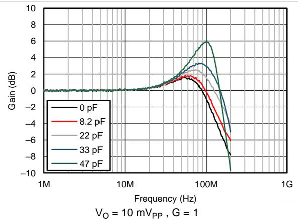
Figure 5. Small-Signal Frequency Response for Various Capacitive Loads
