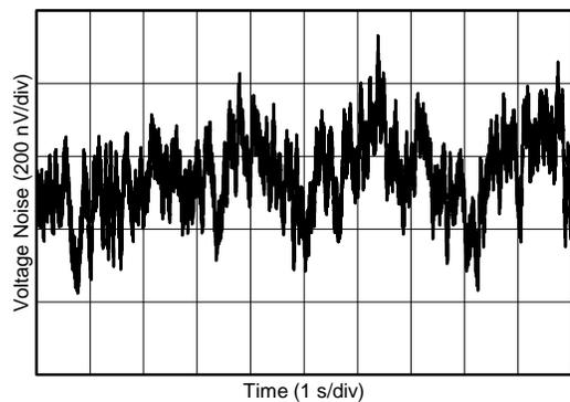
Figure 25. 0.1-Hz to 10-Hz Voltage Noise
