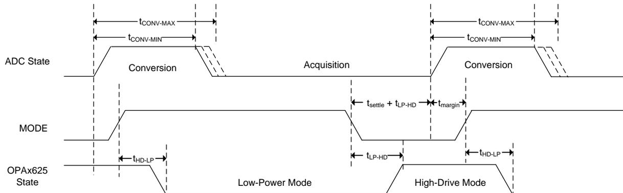
**Figure 71. Simplified Timing Diagram: Power-Scaling Precision Signal Chain**
