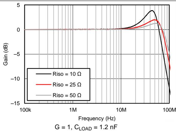
**Figure 14. Series Resistance for Capacitive Load Stability**
