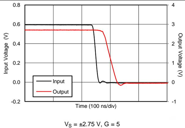
Figure 35. Positive Overload Recovery
