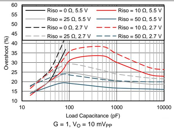
**Figure 15. Overshoot vs Capacitive Load, G = 1**
