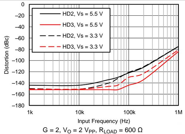
**Figure 19. Distortion vs Frequency for Various Power Supplies**
