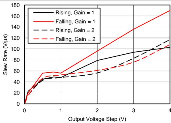
Figure 26. Slew Rate vs Output Step Size
