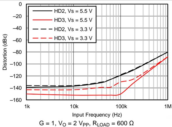
**Figure 18. Distortion vs Frequency for Various Power Supplies**
