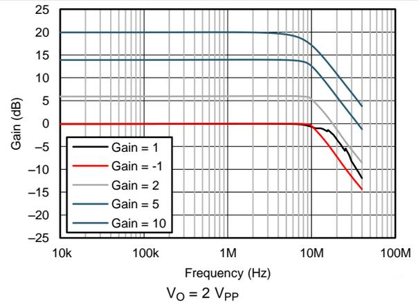
Figure 3. Large-Signal Frequency Response for Various Gains
