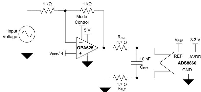
**Figure 73. Single-Supply, 16-Bit, 1-MSPS SAR ADC Driver**
