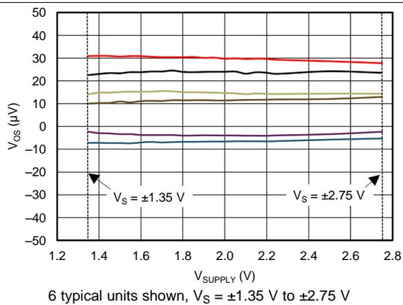
Figure 52. Input Offset Voltage vs Power-Supply Voltage
