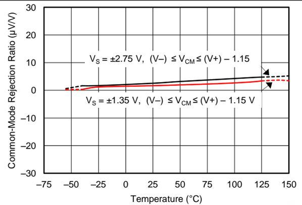
Figure 47. Common-Mode Rejection Ratio vs Temperature
