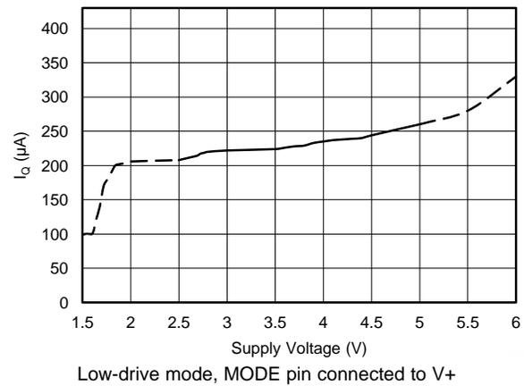
Figure 59. Low-Power Mode Quiescent Current vs Power-Supply Voltage
