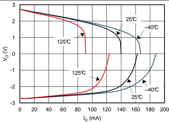
Figure 54. Output Voltage vs Output Current
