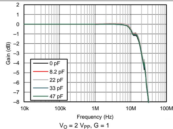
Figure 6. Large-Signal Frequency Response for Various Capacitive Loads
