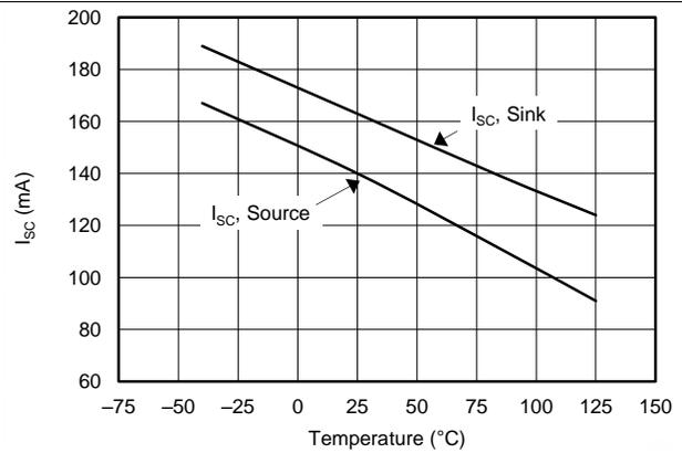
Figure 55. Short-Circuit Current vs Temperature
