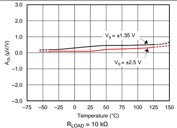
Figure 49. Open-Loop Gain vs Temperature with 10-kΩ Load
