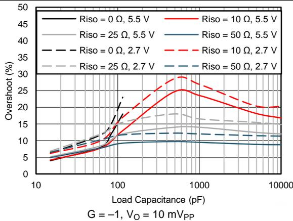
**Figure 16. Overshoot vs Capacitive Load, G = -1**
