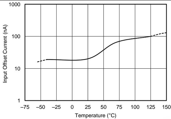
Figure 46. Input Offset Current vs Temperature
