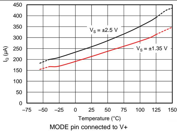
Figure 58. Low-Power Mode Quiescent Current vs Temperature
