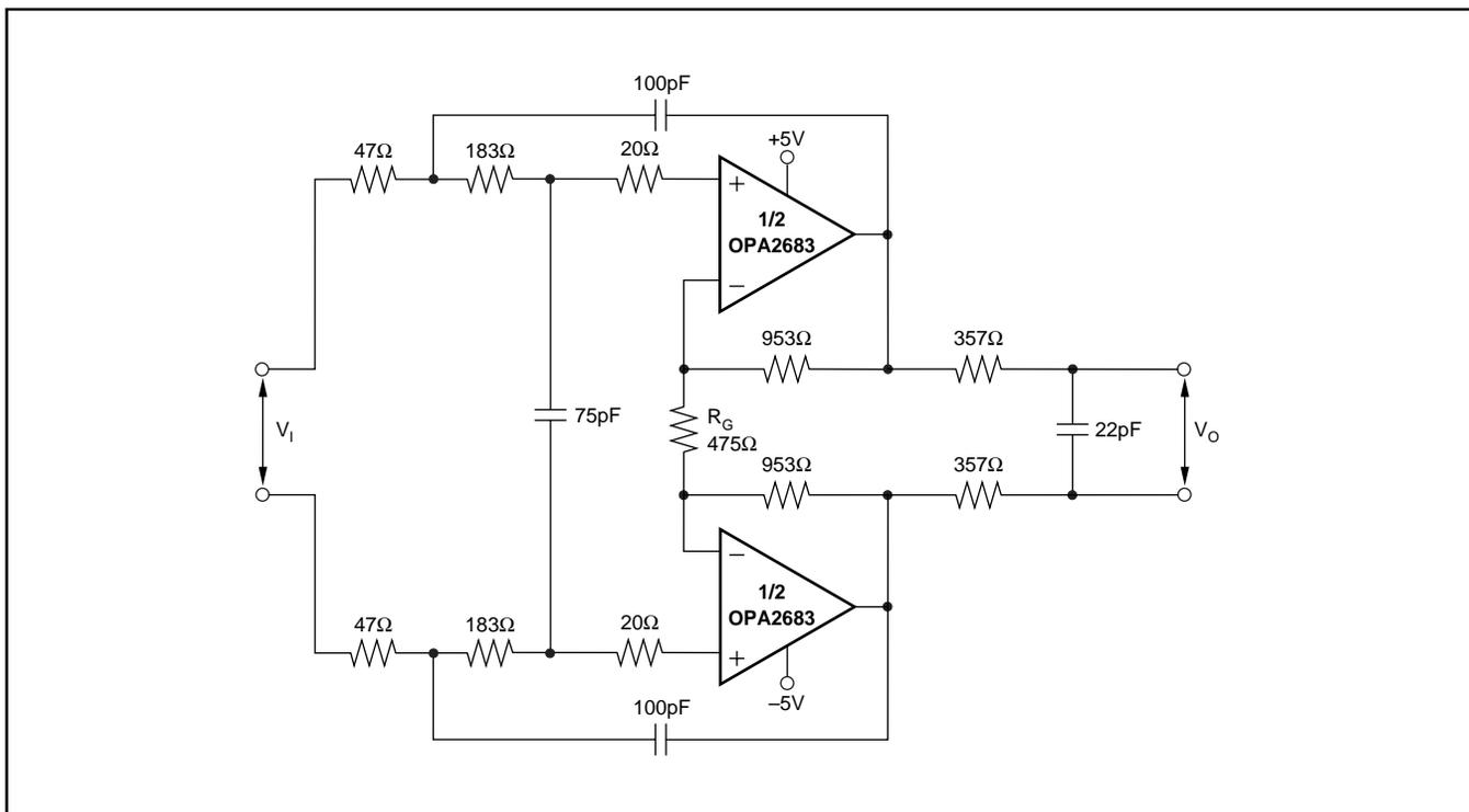
FIGURE 9. Low-Power, Differential I/O, 4th-Order Butterworth Active Filter.
