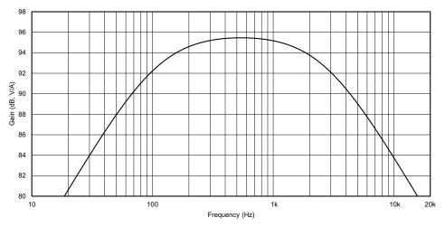
Figure 38. Microphone Preamplifier Transfer Function
