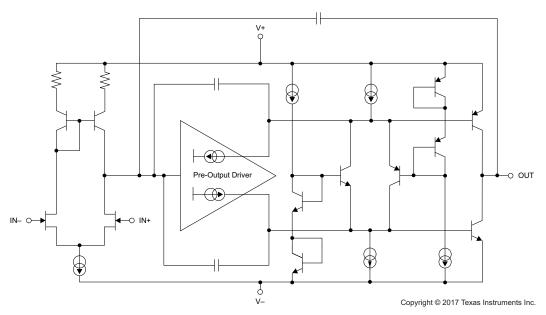
Figure 32. Simplified Internal Schematic
