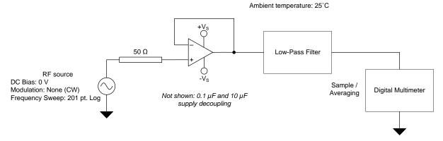
Figure 31. EMIRR IN+ Test Configuration Schematic
