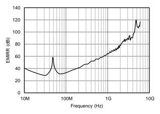
Figure 30. OPA164x-Q1 EMIRR vs Frequency
