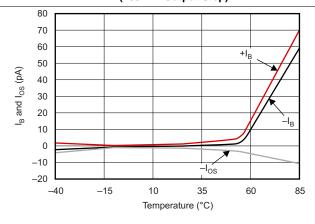
Figure 22.  $I_B$  and  $I_{OS}$  vs Temperature
