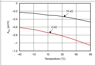
Figure 21. Open-Loop Gain vs Temperature
