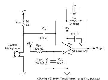
Figure 37. Preamplifier Circuit for Electret Microphones Using a Single Power Supply Voltage
