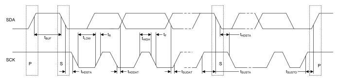
Figure 3. I<sup>2</sup>C Timing Diagram
