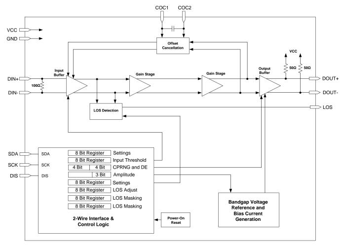
Figure 1. Simplified Block Diagram of the ONET1151P
