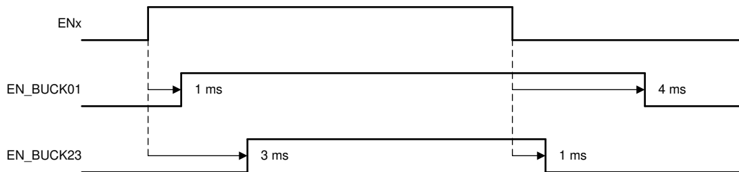
Figure 10. Typical Start-Up and Shutdown Sequencing
