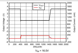
Figure 5-34. Short-Circuit Current vs Time (New Chip)
