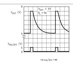
$\label{eq:VOUT} V_{OUT} = 5 V, \ R_L = 5 k \Omega$  Figure 5-52. Turn-Off Waveform (Legacy Chip)
