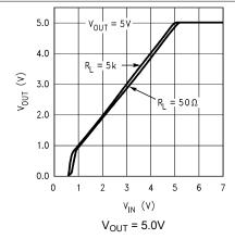
Figure 5-5. Output Voltage vs V<sub>IN</sub> (Legacy Chip)
