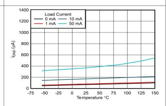
Figure 5-15. Ground Pin Current (I<sub>GND</sub>) vs Temperature (Legacy Chin)
