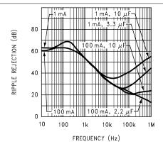
Figure 5-41. Ripple Rejection vs Frequency (Legacy Chip)
