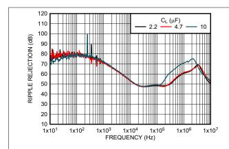
Figure 5-43. Ripple Rejection vs Output Capacitor (C<sub>L</sub>) and Frequency (New Chip)
