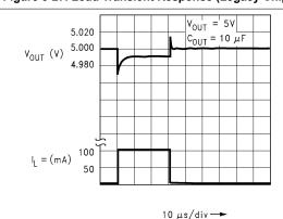
Figure 5-29. Load Transient Response (Legacy Chip)
