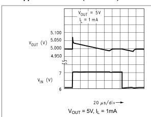
Figure 7-9. Line Transient Response (Legacy Chip)
