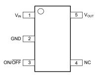
Figure 4-1. DBV Package, 5-Pin SOT-23 (Top View)
