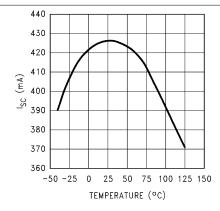
Figure 5-35. Instantaneous Short-Circuit Current vs Temperature (Legacy Chip)
