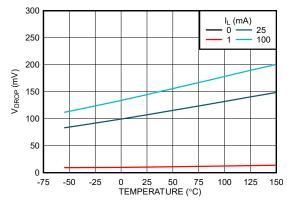
**Dropout Voltage vs Temperature (New Chip)**
