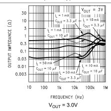
Figure 5-40. Output Impedance vs Frequency (Legacy Chip)
