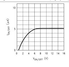
Figure 5-54. ON/OFF Pin Current vs V<sub>ON/OFF</sub> (Legacy Chip)
