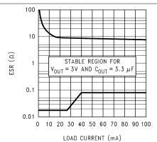
$\label{eq:VOUT} V_{OUT} = 3.0V, \, C_{OUT} = 3.3 \mu F$  Figure 7-5. 3.0V, 3.3 $\mu F$  ESR Curves (Legacy Chip)
