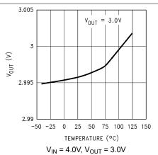
Figure 5-3. Output Voltage vs Temperature (Legacy Chip)
