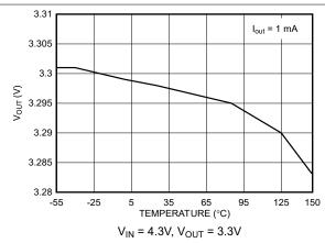
Figure 5-4. Output Voltage vs Temperature (New Chip)
