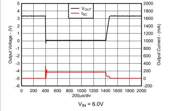
Figure 5-32. Short-Circuit Current vs Time (New Chip)
