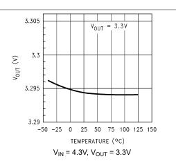
Figure 5-2. Output Voltage vs Temperature (Legacy Chip)
