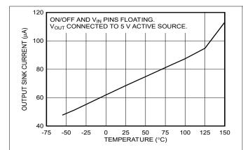
Figure 5-49. Output Reverse Leakage vs Temperature (New Chip)
