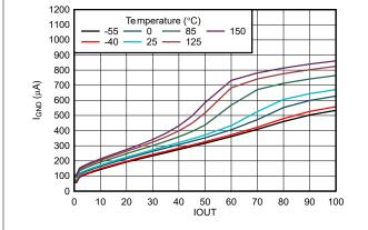
Figure 5-17. Ground Pin Current (I<sub>GND</sub>) vs Load Current (Legacy Chip)
