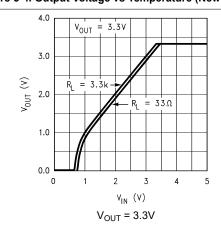
Figure 5-6. Output Voltage vs V<sub>IN</sub> (Legacy Chip)
