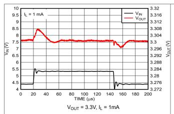
Figure 5-25. Line Transient Response (New Chip)
