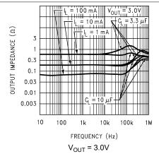
Figure 5-39. Output Impedance vs Frequency (Legacy Chip)
