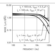
Figure 5-44. Output Noise Density vs Frequency (Legacy Chip)
