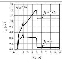
$V_{OUT}$  = 5V,  $R_L$  =  $\infty$  and  $R_L$  =  $5k\Omega$
