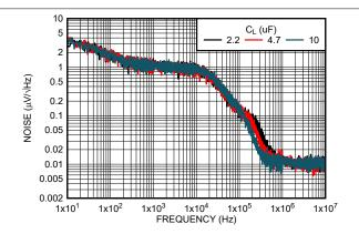
Figure 5-46. Output Noise Density vs Output Capacitor ( $C_L$ )
