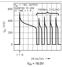
Figure 5-33. Short-Circuit Current vs Time (Legacy Chip)
