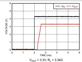
Figure 5-51. Turn-On Waveform (New Chip)
