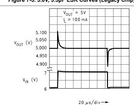
Figure 7-7. Line Transient Response (Legacy Chip)
