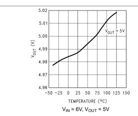
Figure 5-1. Output Voltage vs Temperature (Legacy Chip)
