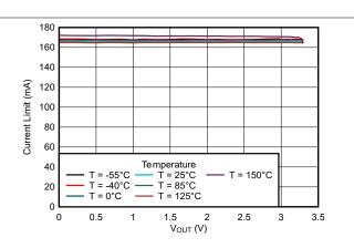
Figure 5-38. Short-Circuit Current vs Output Voltage (V<sub>OUT</sub>) (New Chip)
