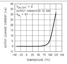
Figure 5-47. Input-to-Output Leakage vs Temperature (Legacy Chip)
