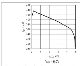
Figure 5-37. Short-Circuit Current vs Output Voltage (V<sub>OUT</sub>) (Legacy Chip)
