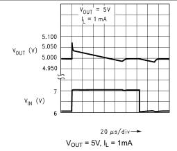
Figure 5-24. Line Transient Response (Legacy Chip)
