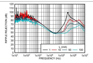
Figure 5-42. Ripple Rejection vs Load Current (I<sub>L</sub>) and Frequency (New Chip)
