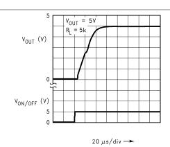
Figure 5-50. Turn-On Waveform (Legacy Chip)
