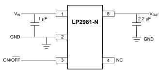
\*The ON/OFF input must be actively terminated. Tie to V<sub>IN</sub> if this function is not to be used. Minimum output capacitance is shown to provide stability over full load current range. More capacitance provides superior dynamic performance and additional stability margin (see the Recommended Capacitor Types section).
