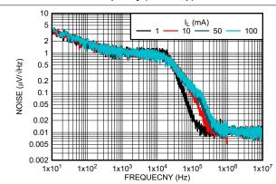
Figure 5-45. Output Noise Density vs Load Current ( $I_L$ )
