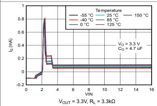
Figure 5-21. Input Current vs Input Voltage (V<sub>IN</sub>) (New Chip)
