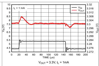
Figure 7-10. Line Transient Response (New Chip)
