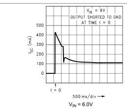
Figure 5-31. Short-Circuit Current vs Time (Legacy Chip)
