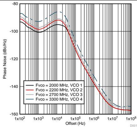
Figure 4. Closed Loop Noise for Narrower Bandwidth Filter
