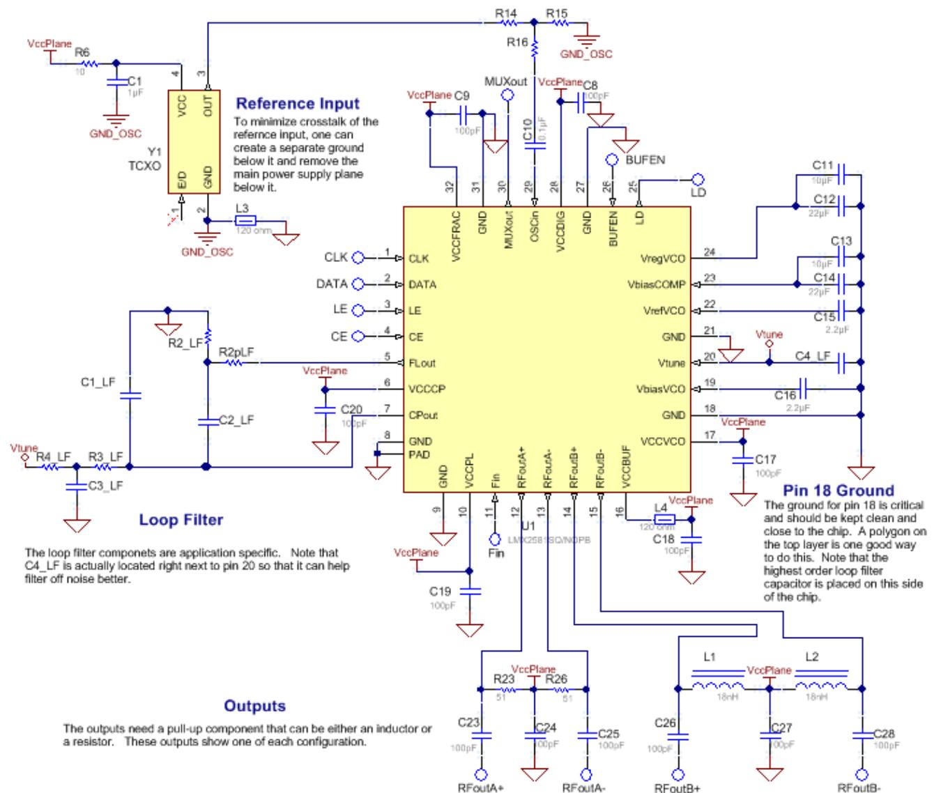
Figure 21. Typical Schematic
