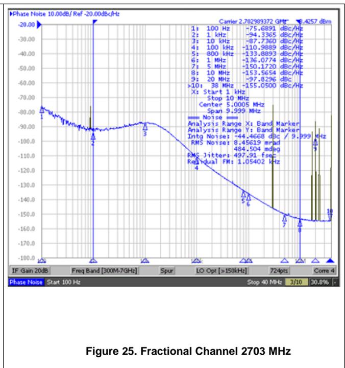
Figure 25. Fractional Channel 2703 MHz
