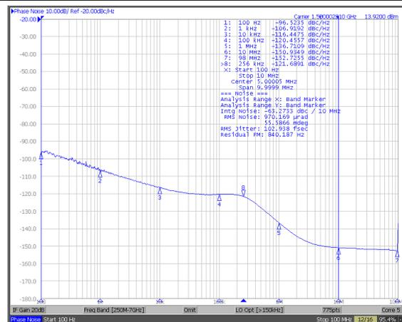
Figure 23. Measured Plot
