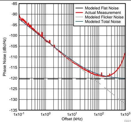
Figure 2. Measurement of PLL Figure of Merit and Normalized 1/f Noise
