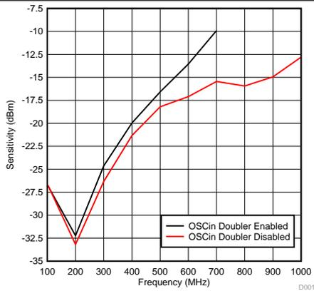
Figure 12. OSCin Input Sensitivity
