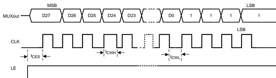
**Figure 19. Timing for Readback, Holding LE High**
