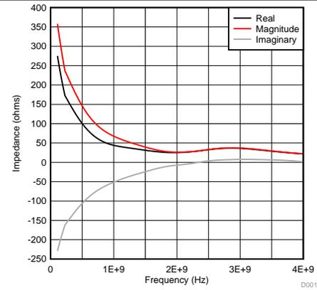
Figure 11. Impedance of External VCO Input (Fin) Pin
