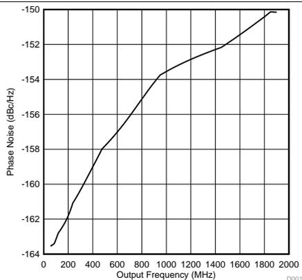
Figure 6. VCO Output Divider Noise Floor vs. Frequency
