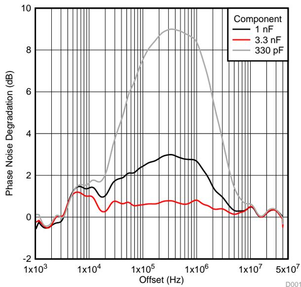
Figure 17. Vtune Capacitor Impact on VCO Phase Noise
