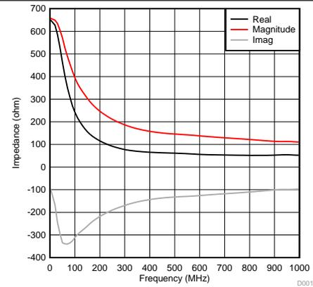
Figure 13. OSCin Input Impedance
