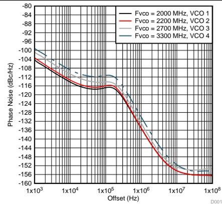
Figure 5. Closed Loop Noise for Wider Bandwidth
