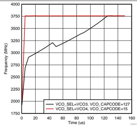
Figure 7. VCO Digital Calibration Time
