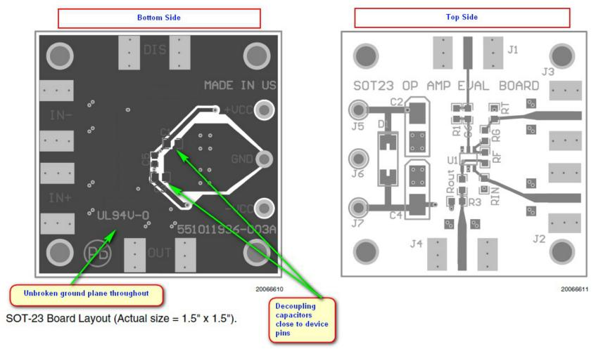
Figure 20. SOT-23 Board Layout Example
