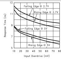
Figure 11. Propagation Delay vs. Input Overdrive
