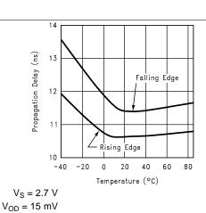
Figure 8. Propagation Delay vs. Temperature
