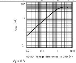
Figure 7. Sinking Current vs. Output Voltage
