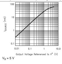
Figure 4. Sourcing Current vs. Output Voltage
