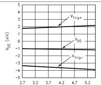
Figure 2.  $V_{OS}$  vs. Supply Voltage
