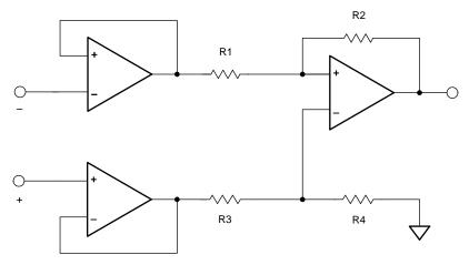
Figure 32. Rail-to-Rail Instrumentation Amplifier
