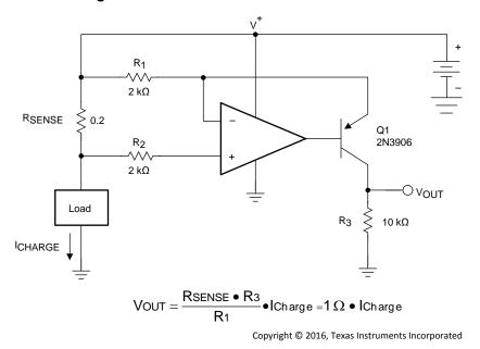
Figure 33. High-Side, Current-Sensing Schematic
