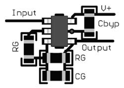
Figure 35. SOT-23 Layout Example
