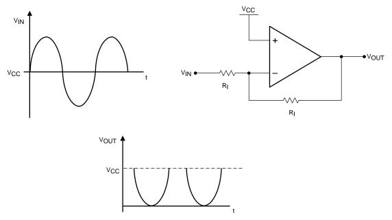
Figure 31. Half-Wave Rectifier With Negative-Going Output Referenced to V<sub>CC</sub>
