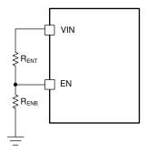
Figure 8-3. System UVLO by Enable Divider
