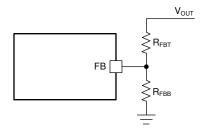
Figure 8-2. Output Voltage Setting
