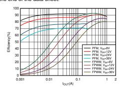
Efficiency versus Output Current  $V_{OUT} = 5 V$ , 2.1MHz
