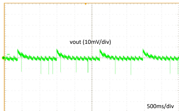
LMR43620MB5 V_{OUT} = 5\text{ V} f_{SW} = 1\text{ MHz (auto)} Fixed V_{IN} = 24\text{ V} I_{OUT} = \text{Open}
