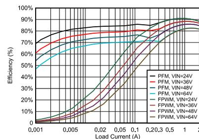
**Efficiency vs Output Current V<sub>OUT</sub> = 5V, 400kHz**
