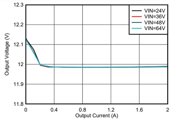
LMR38020-Q1  $V_{OUT} = 12\text{ V}$  400 kHz
