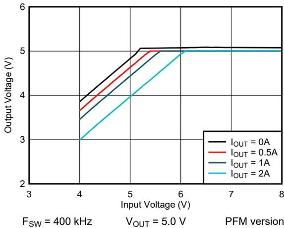
Figure 6-3. 5-V Dropout
