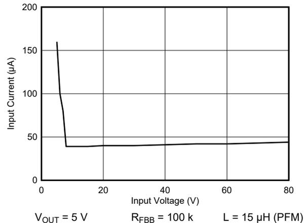
Figure 6-2. No Load Input Current vs Input Voltage
