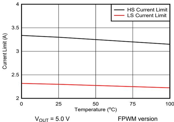
Figure 6-5. High-Side and Low-Side Current Limit vs Temperature
