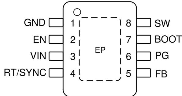
Figure 5-1. DDA Package, 8-Pin HSOIC (Top View)
