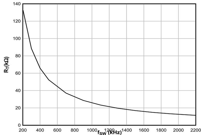
Figure 7-4. R<sub>T</sub> Versus Frequency CurveTable 7-1. Typical Frequency Setting R<sub>T</sub> Resistance
