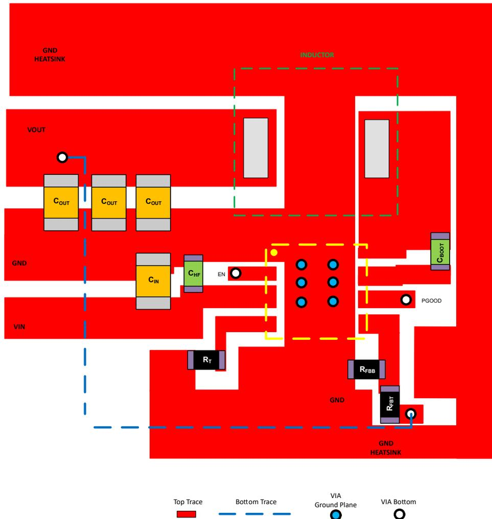
Figure 8-16. Example Layout for HSOIC (DDA) Package
