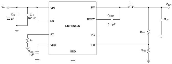
Figure 9-18. Schematic for Typical Application Curves
