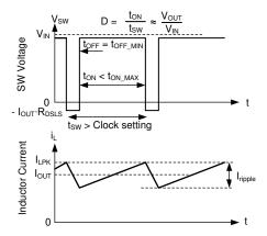
Switching waveforms while in dropout. Inductor current takes longer than a normal clock to reach the desired peak value. As a result, frequency drops. This frequency drop is limited by  $t_{\text{ON-MAX}}$ .
