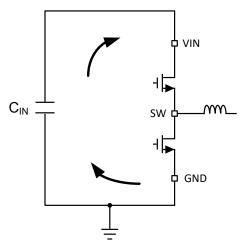
Figure 9-19. Current Loops with Fast Edges
