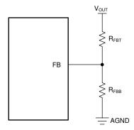
Figure 8-6. Setting Output Voltage for Adjustable Output Variant
