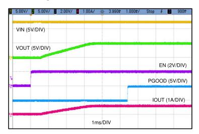
Figure 8-3. Enable Start-up  $V_{IN}$  = 12 V,  $V_{OUT}$  = 5 V,  $I_{OUT}$  = 600 mA
