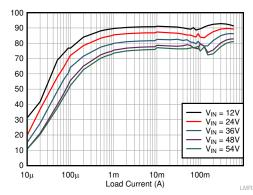
Efficiency versus Output Current V<sub>OUT</sub> = 5 V (Fix), 1 MHz
