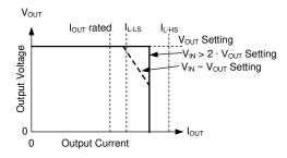
Figure 8-11. Output Voltage versus Output Current
