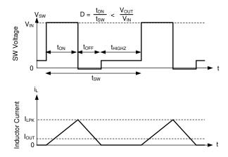
In auto mode, the low-side device is turned off after SW node current is near zero. As a result, after output current is less than half of what inductor ripple is in CCM, the part operates in DCM which is equivalent to the statement that diode emulation is active.
