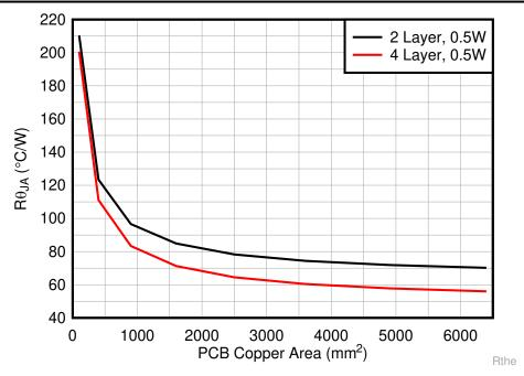
Figure 9-3. R<sub>0,JA</sub> versus PCB Copper Area for the VQFN (RPE) Package
