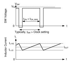
Figure 8-10. Current Limit Waveforms
