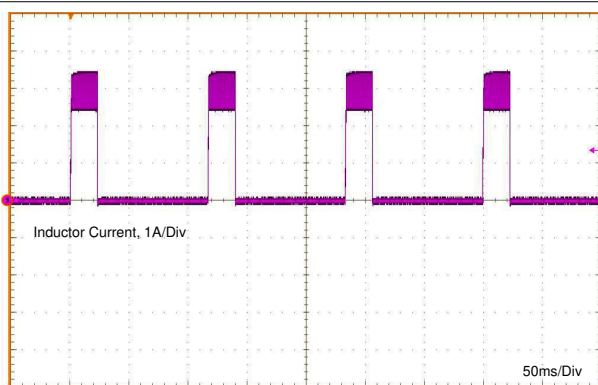
Figure 8-5. Inductor Current Burst in Short-Circuit Mode
