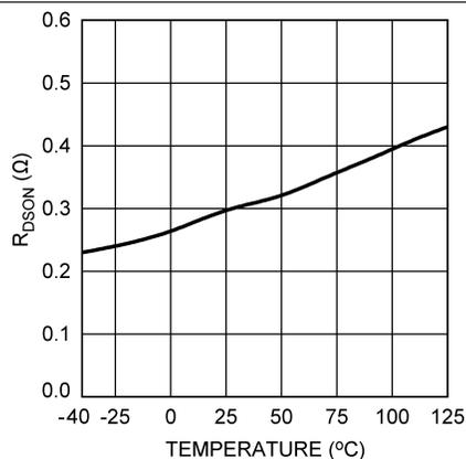
Figure 12.  $R_{DS(on)}$  vs Temperature
