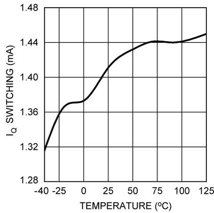
**Figure 13. I<sub>Q</sub> Switching vs Temperature**
