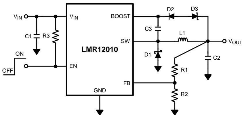
Figure 19.  $V_{BOOST}$  Derived From Series Zener Diode ( $V_{OUT}$ )
