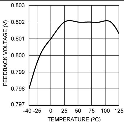
Figure 11.  $V_{FB}$  vs Temperature
