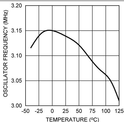
Figure 8. Oscillator Frequency vs Temperature - "Y"
