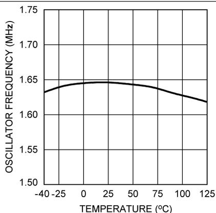
Figure 7. Oscillator Frequency vs Temperature - "X"
