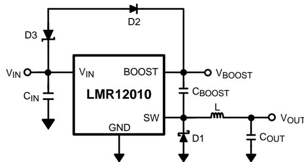
**Figure 16. Zener Reduces Boost Voltage From  $V_{IN}$**
