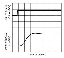
Figure 23. Settling Time (Rising Edge) at V<sub>S</sub> = 3.3 V LMP8602 and LMP8602-Q1
