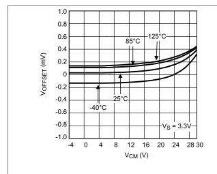
Figure 1.  $V_{OS}$  vs  $V_{CM}$  at  $V_{S}$  = 3.3 V
