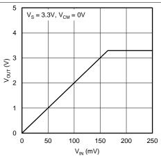
Figure 51. Output Voltage vs VIN
