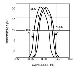
Figure 43. Gain Error Distribution at  $V_S = 3.3 \text{ V}$ , 5000 Parts LMP8602 and LMP8602-Q1
