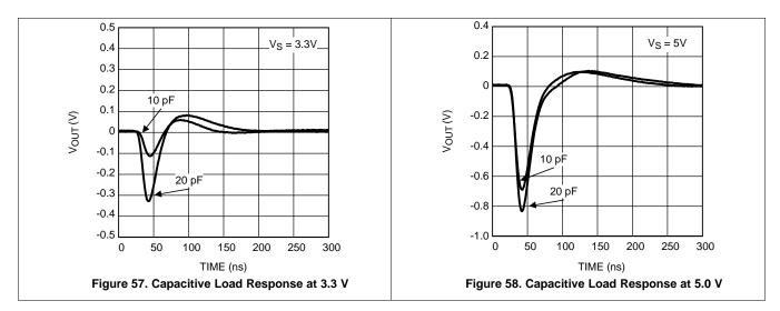
These figures can be used to estimate the disturbance that will be caused when driving a switched capacitive load. To minimize the error signal introduced by the sampling that occurs on the ADC input, place an additional RC filter between the LMP860x or LMP860x-Q1 and the ADC, as illustrated in Figure 59.
