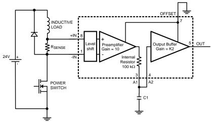
$R_{SENSE} = 0.01 \Omega$ , K2 = 2,  $V_{OUT} = 0.2 V/A$
