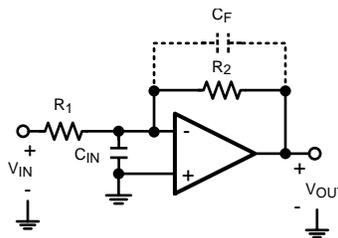
$$A_V = - \frac{V_{OUT}}{V_{IN}} = - \frac{R_2}{R_1}$$
