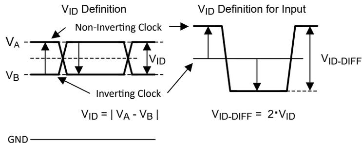
Figure 6-7. Two Different Definitions for Differential Input Signals
