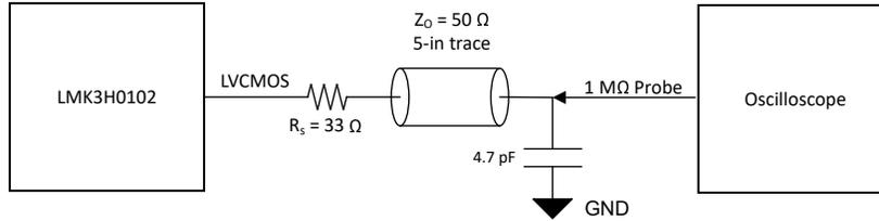
Figure 6-1. LVC MOS Output Configuration During Device Test
