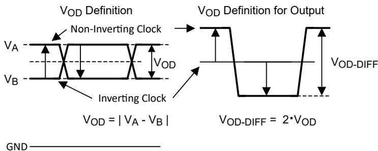
Figure 6-8. Two Different Definitions for Differential Output Signals
