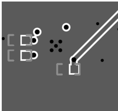
Figure 9-9. PCB Layout Example for LMK3H0102, Bottom Layer
