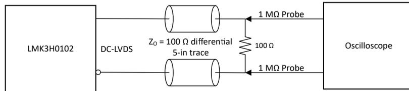
Figure 6-3. DC-LVDS Output Configuration During Device Test
