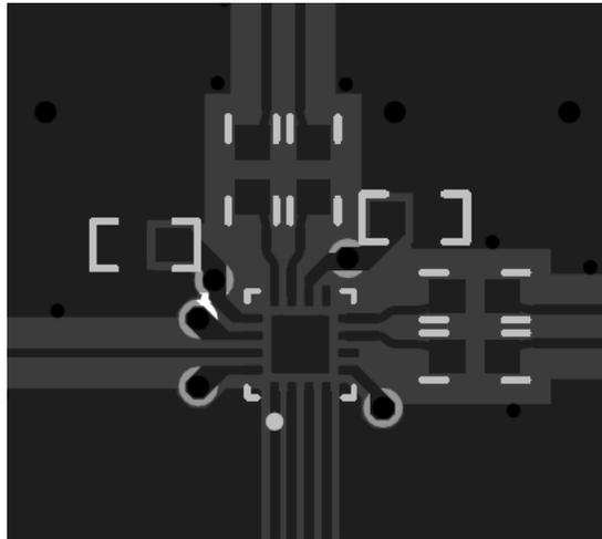
Figure 9-8. PCB Layout Example for LMK3H0102, Top Layer
