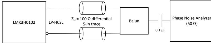
Figure 6-6. PCIe Test Configuration Using Phase Noise Analyzer
