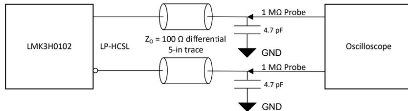
Figure 6-4. LP-HCSL Output Configuration During Non-PCIe Device Test
