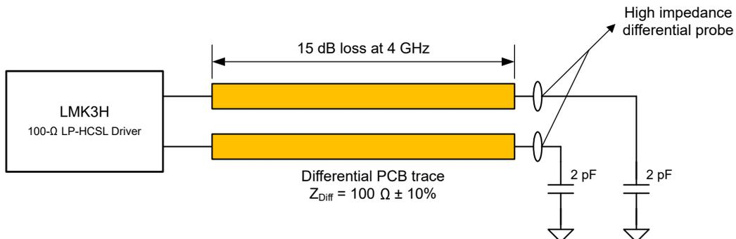
Figure 6-5. LP-HCSL Output Configuration During PCIe Device Test
