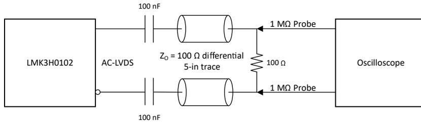
Figure 6-2. AC-LVDS Output Configuration During Device Test
