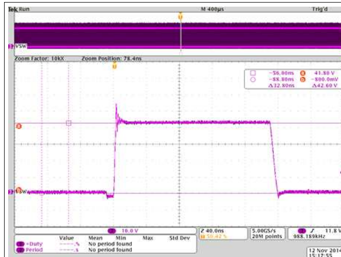
Figure 12. SW Node Behavior Showing the Dead Time
