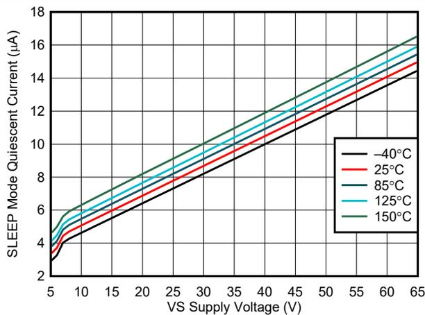
Figure 6-3. SLEEP Mode Current vs Supply Voltage
