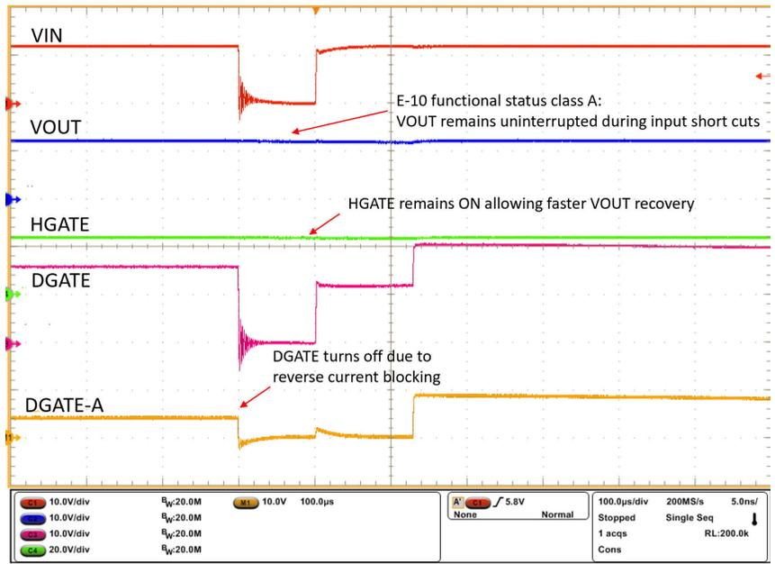
**Figure 9-4. Input Micro-Short - LV124 E10 TC 2 100 μs**
