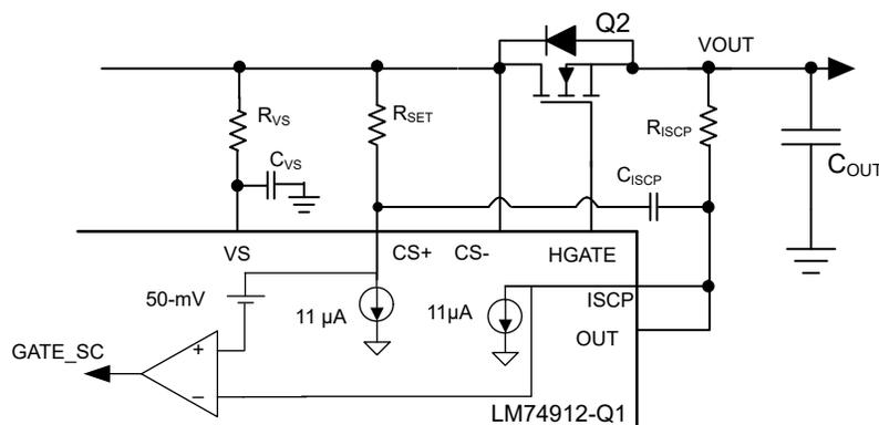
**Figure 8-4. Short Circuit Protection With De-glitch Filter**
