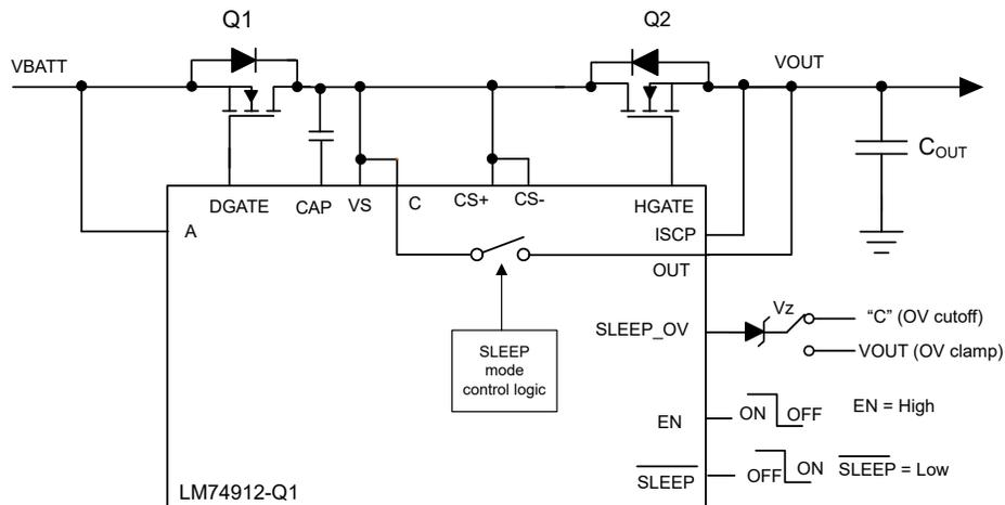
**Figure 8-7. Extending Overvoltage Threshold in SLEEP Mode**
