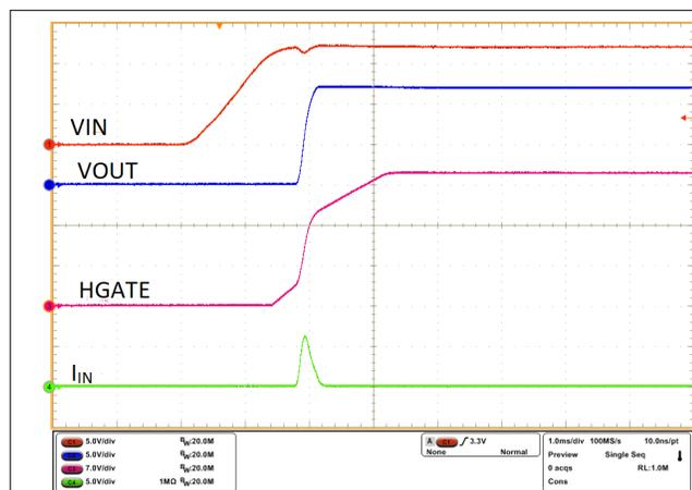
**Figure 9-5. Startup 12 V with EN Pulled to VS**
