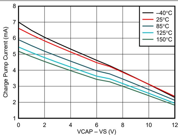
Figure 6-5. Charge Pump V-I Characteristics at VS ≥ 12 V
