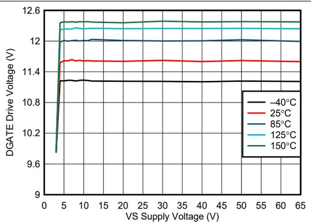
Figure 6-6. DGATE Drive Voltage vs Supply Voltage
