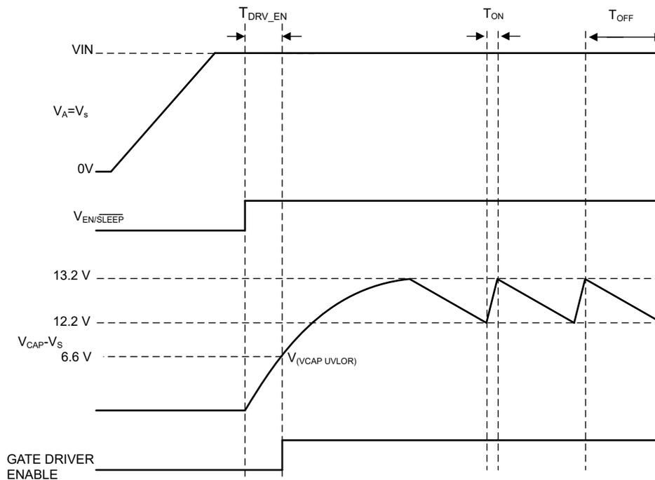
Figure 8-1. Charge Pump Operation
