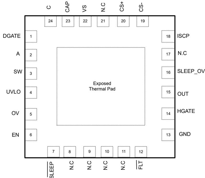
Figure 5-1. RGE Package, 24-Pin VQFN (Transparent Top View)
