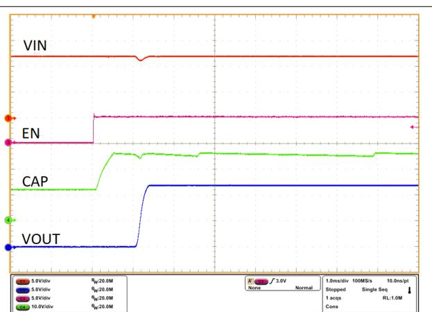
**Figure 9-6. Startup with EN Going Low to High**
