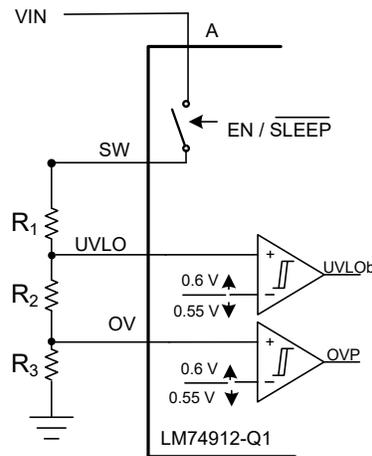
**Figure 8-5. Programming Overvoltage Threshold and Battery Sensing**
