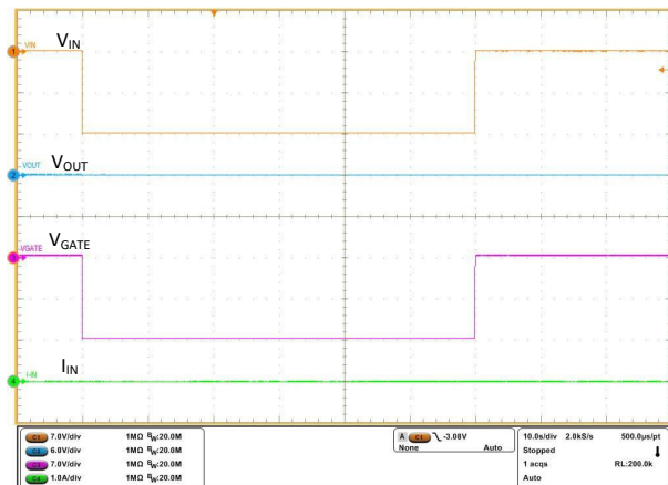
Figure 9-9. Reverse Input Voltage -14\text{ V} for 60 s
