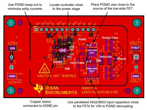
Figure 8-47. PCB Top Layer - High Density, Single-sided Design
