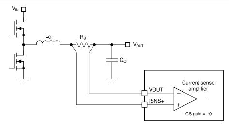
Figure 7-4. Shunt Current Sensing Implementation
