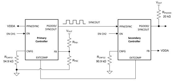
Figure 7-7. Schematic Configured for Single-Output Dual-Phase Operation
