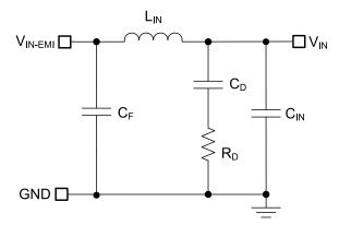
Figure 8-2. Passive π-Stage EMI Filter for Buck Regulator
