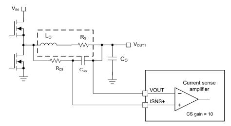
Figure 7-5. Inductor DCR Current Sensing Implementation
