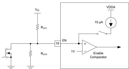
Figure 7-2. Programmable Input Voltage UVLO Turn-On
