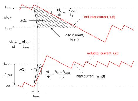
Figure 8-1. Load Transient Response Representation Showing C<sub>OUT</sub> Charge Surplus or Deficit
