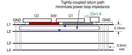
Figure 8-49. PCB Stack-up Diagram With Low L1-L2 Intra-layer Spacing <sup>1</sup>
