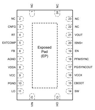
Figure 5-1. 24-Pin VQFN RGY Package With Wettable Flanks, LM5148QRGYRQ1 (Top View)
