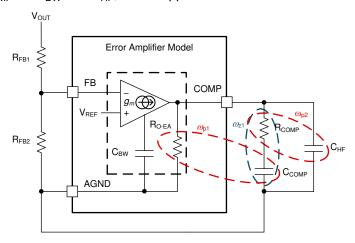
Figure 8-3. Error Amplifier and Compensation Network
