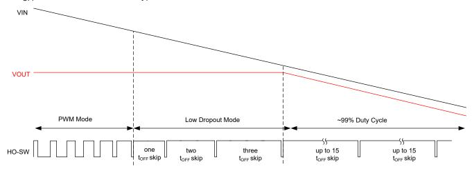
Figure 7-1. Dropout Mode Operation
