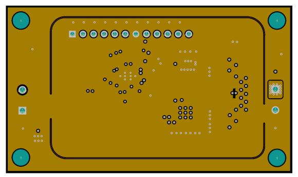
Figure 8-48. Layer 2 Full Ground Plane Directly Under the Power Components
