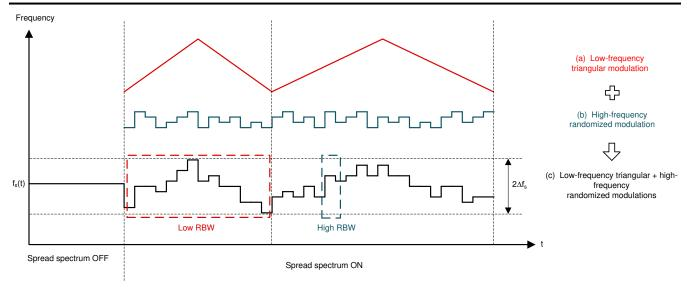
Figure 7-3. Dual Random Spread Spectrum Implementation
