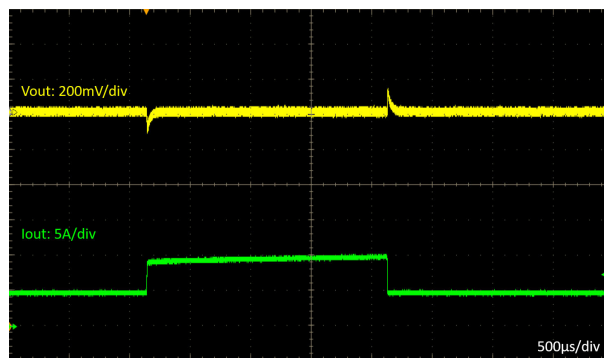
Figure 7-12. Load Transient, 5A to 10A
