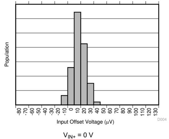
**Figure 6-4. Input Offset Voltage Production Distribution (INA381A4-Q1)**
