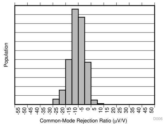
**Figure 6-6. Common-Mode Rejection Ratio Production Distribution (INA381A1-Q1)**
