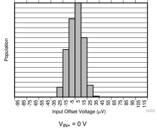
**Figure 6-2. Input Offset Voltage Production Distribution (INA381A2-Q1)**
