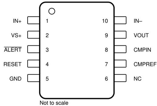
**Figure 5-1. DGS Package 10-Pin VSSOP Top View**
