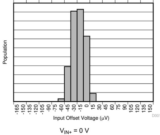
**Figure 6-1. Input Offset Voltage Production Distribution (INA381A1-Q1)**
