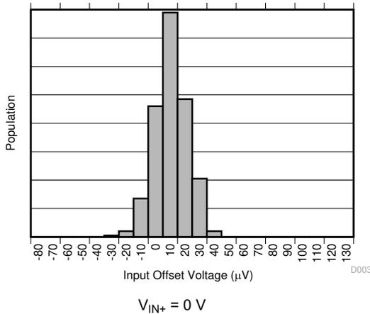
**Figure 6-3. Input Offset Voltage Production Distribution (INA381A3-Q1)**
