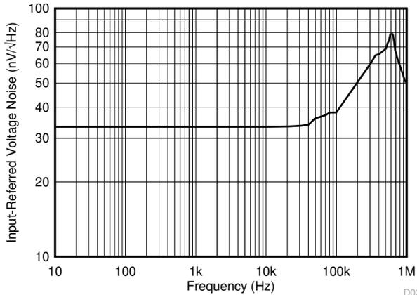
**Figure 6-25. Input-Referred Voltage Noise vs. Frequency (INA381A3-Q1 Devices)**
