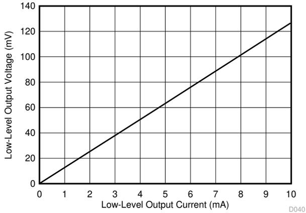
**Figure 6-37. Low-Level Output Voltage vs. Low-Level Output Current**
