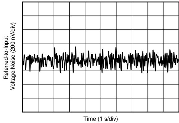
**Figure 6-26. 0.1-Hz to 10-Hz Voltage Noise (Referred-to-Input)**
