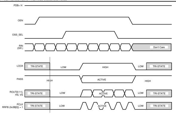
Figure 4-8. Output State (Setup and Hold) Times
