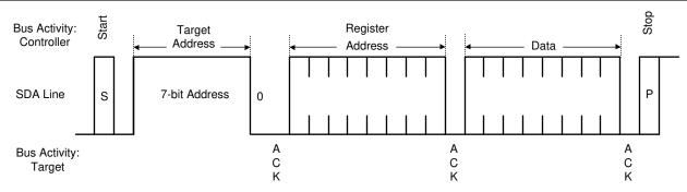
Figure 5-9. Serial Control Bus — WRITE
