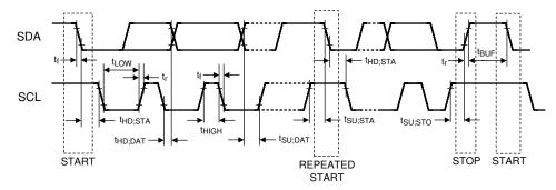
Figure 4-4. I2C Serial Control Bus Timing
