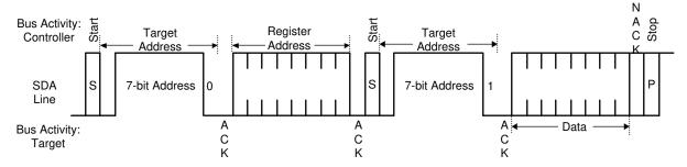
Figure 5-8. Serial Control Bus — READ
