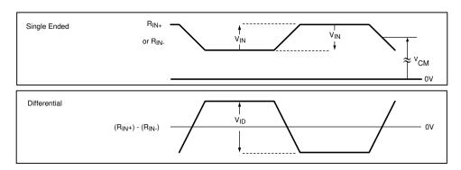
Figure 4-2. FPD-Link III Receiver  $V_{\text{ID}}, \, V_{\text{IN}}, \, V_{\text{CM}}$
