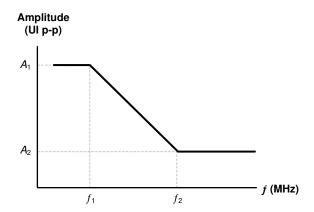
Figure 5-3. Input Jitter Tolerance Plot
