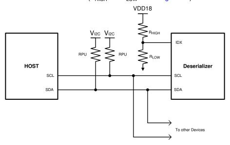
Figure 5-6. Serial Control Bus Connection
