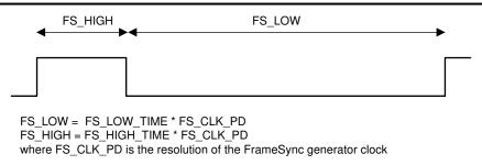
Figure 5-5. Internal FrameSync Signal
