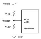
Figure 5-2. Strap Pin Connection Diagram
