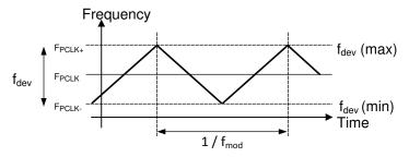
Figure 4-9. Spread Spectrum Clock Output Profile
