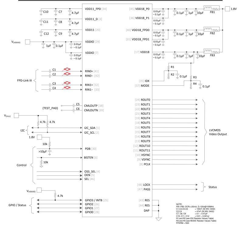
Figure 6-4. Typical Connection Diagram STP
