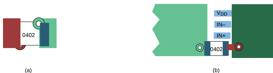
Figure 21. Typical Decoupling Capacitor Layouts
