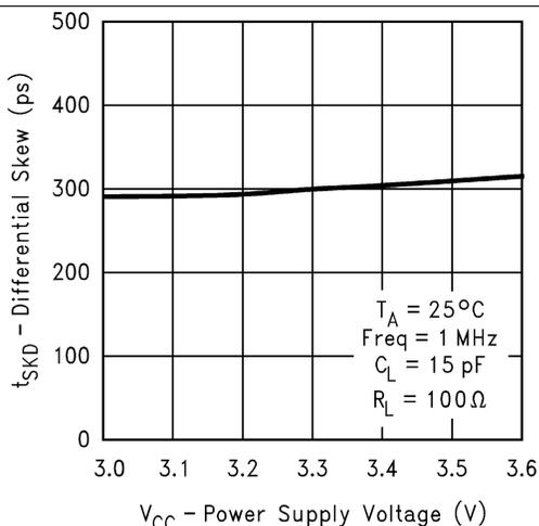
**Figure 11. Differential Skew vs Power Supply Voltage**
