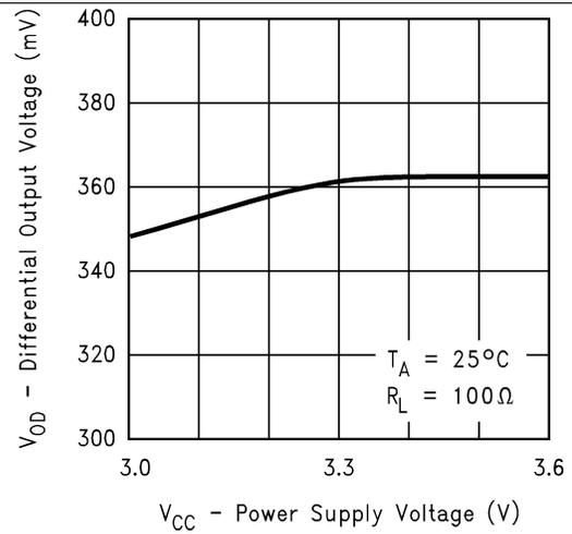
**Figure 4. Differential Output Voltage vs Power Supply Voltage**
