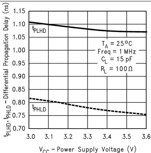
**Figure 9. Differential Propagation Delay vs Power Supply Voltage**
