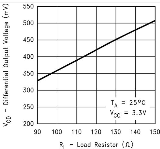
**Figure 5. Differential Output Voltage vs Load Resistor**
