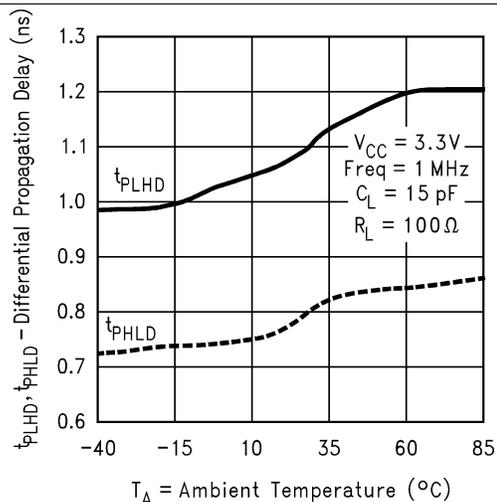
**Figure 10. Differential Propagation Delay vs Ambient Temperature**
