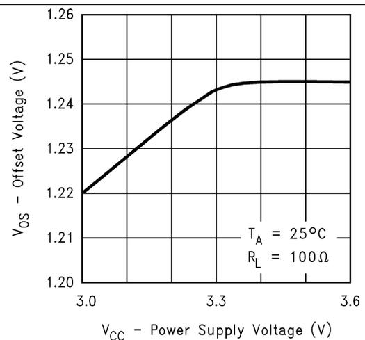
**Figure 6. Offset Voltage vs Power Supply Voltage**
