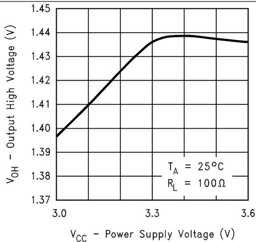
**Figure 1. Output High Voltage vs Power Supply Voltage**
