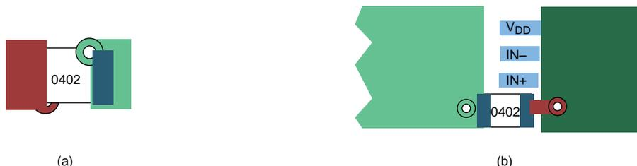
Figure 30. Typical Decoupling Capacitor Layouts
