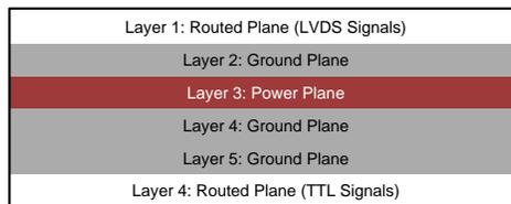
**Figure 27. Six-Layer PCB**
