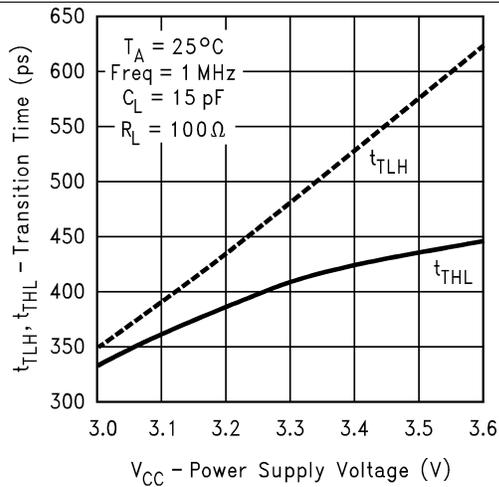
**Figure 13. Transition Time vs Power Supply Voltage**
