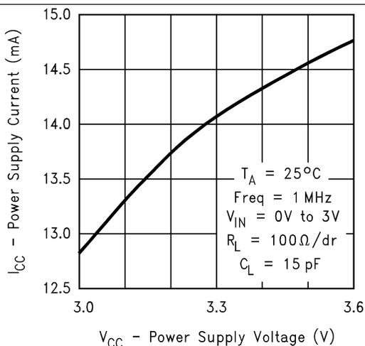
**Figure 7. Power Supply Current vs Power Supply Voltage**
