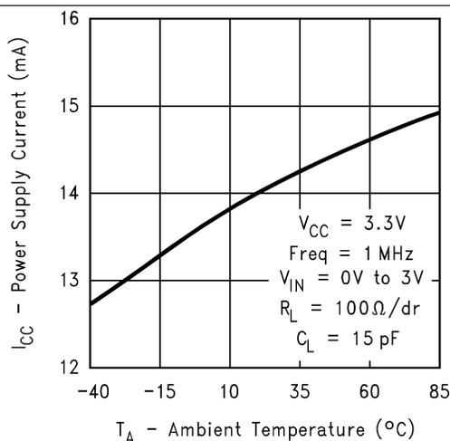
**Figure 8. Power Supply Current vs Ambient Temperature**
