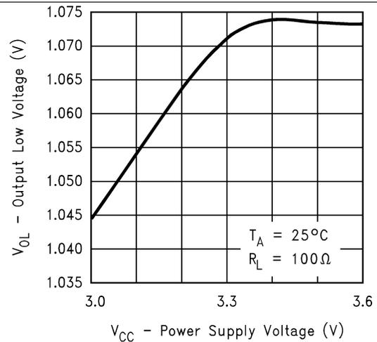
**Figure 2. Output Low Voltage vs Power Supply Voltage**
