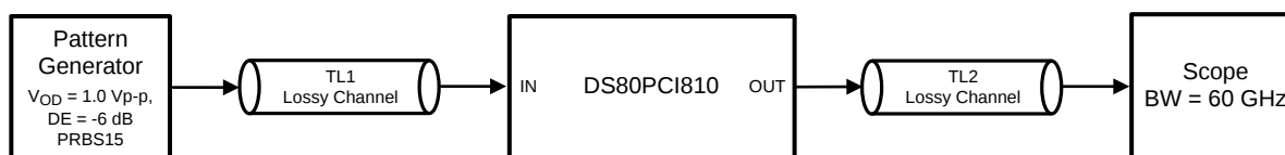
Figure 10. Test Setup Connections Diagram
