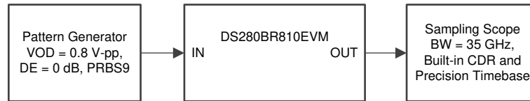
Figure 11. Minimal Rx/Tx Channel Test Setup
