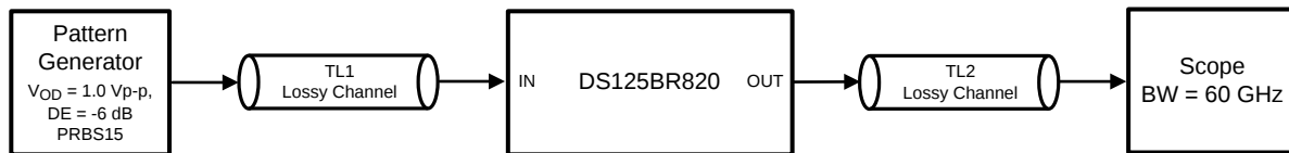
Figure 10. Test Setup Connections Diagram
