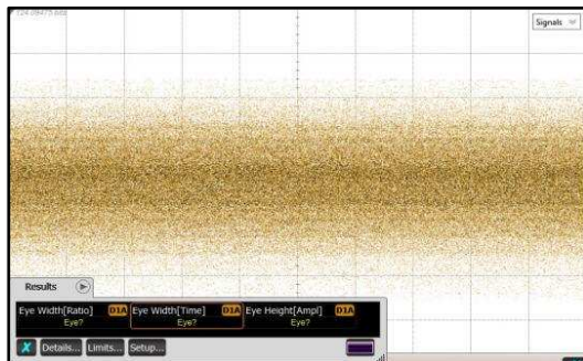
Figure 27. TL = 7-Meter 30-AWG 100 \Omega Twin-Axial Cable, No Repeater, 10.3125 Gbps
