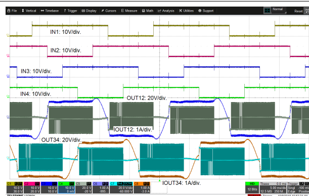
Figure 8-9. Stepper Motor Half-Step Operation With Off-State as Brake
